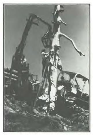
"Chains padded with canvas and suspended from the selfloader were secured around the base and a third of the way up the trunk."
