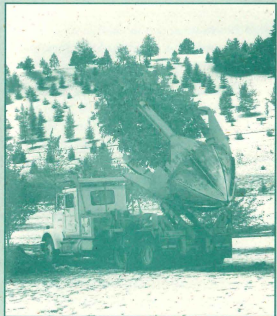
Justin Bowen, Lone Pine Tree Service, Rexburg, ID, guides a 90" "Big John" tree spade in moving a specimen 'Urbanite' ash for the Public Utilities Executives' Course grove in the Arboretum after our first snowfall. R.J. Naskali photo, October 19, 1996.
