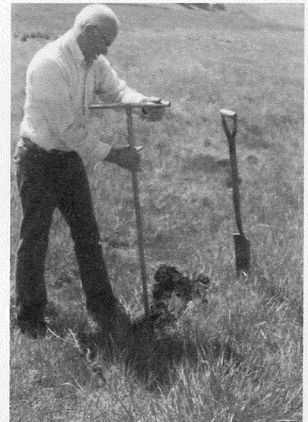
Professor Maynard Fosberg drills a soil core to find the depth of intact, impervious 'blue clay' for setting the depth of pond grading for the dams. June, 1986.
