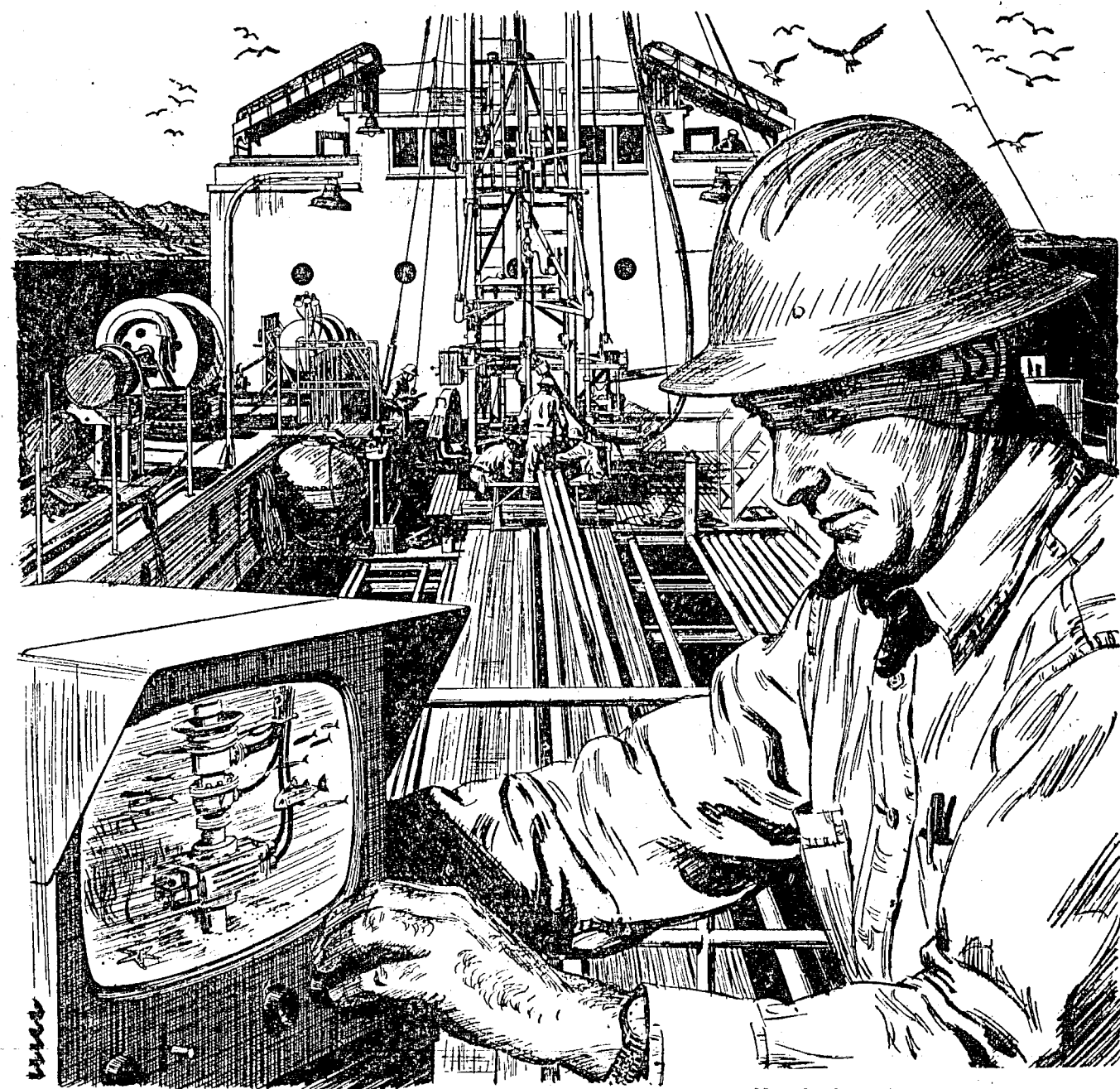
Navy landing ship converted by Standard for off-shore oil search. A 55-foot drilling mast is poised over circular 10-foot-wide opening from deck through bottom.
