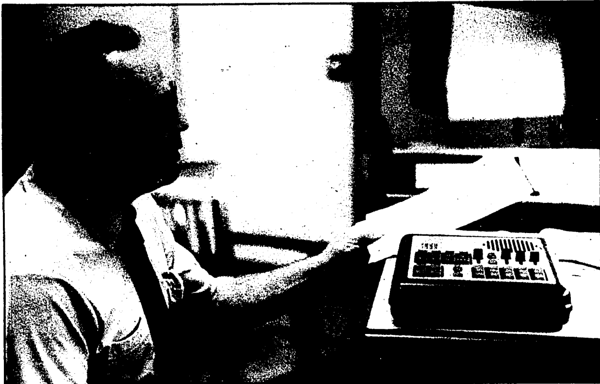
Richard Beck, Associate Dean of Libraries, demonstrates the Kurzweil Reader. This device will automatically read aloud in a synthetic voice the English language whether printed or type written. Photo Bureau/Tina Old-Mouse.
