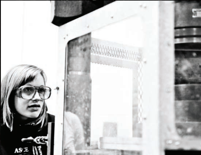
DeAnn Brown tests a concrete core's merit under tons of pressure. Sample cores are broken and analyzed as the team develops stronger, lighter concrete.
