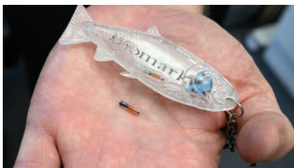
ABOVE: A LIFE-SIZED PLASTIC REPRESENTATION OF A JUVENILE SALMON WITH THE RADIO TAGGING DEVICES USED BY CAUDILL AND HIS TEAM.
