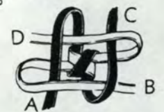
Loop B over A and through C strand loop. Pull tight to form square as in Fig. 6.
