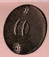
One head of each drum to be fitted with a manhole 12 inches by 16 inches. The heads to be hydraulic forged at a single heat, the manhole to be flanged inward, and the face to be turned off true.
