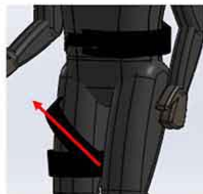
Figure 2. Model of orthosis design. Red arrow shows where the force is applied to rotate the hip.
