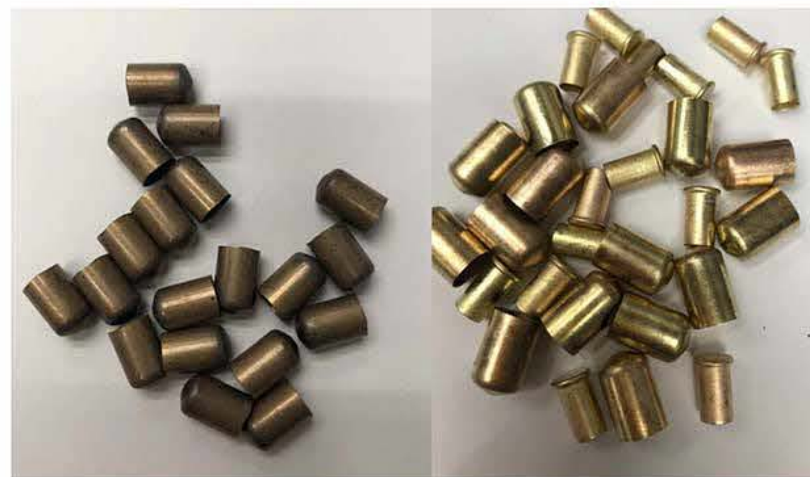
Figure 2: Part on the left are annealed under atmospheric air while parts on the right are annealed under an exothermic atmosphere.
