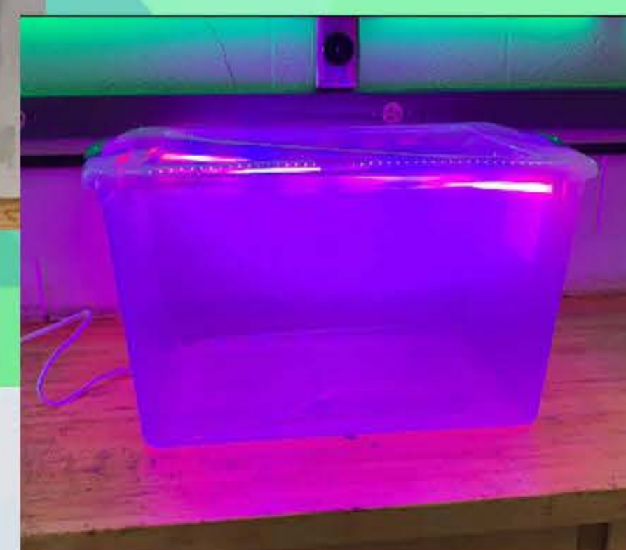
(Above) The tub used to grow algae. The purple light was not ideal for algae growth. White light worked better.
