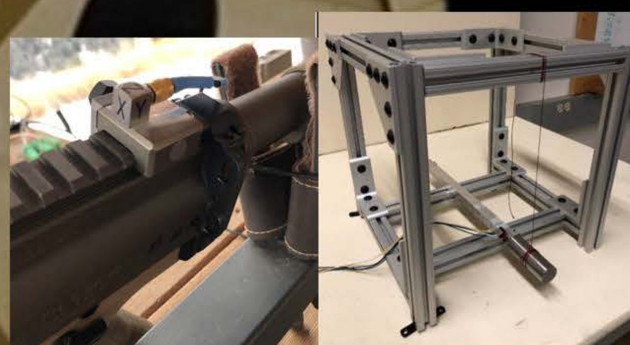
Capturing acceleration data with accelerometer on rifle rail.
