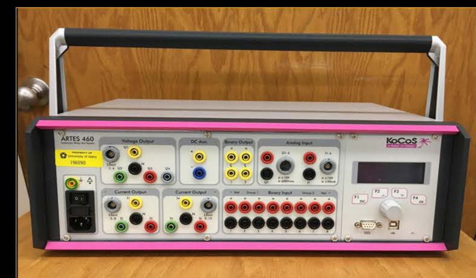
KoCoS ARTes 460 The KoCoS is used to apply voltage and current to devices for accurate measurement and testing.
