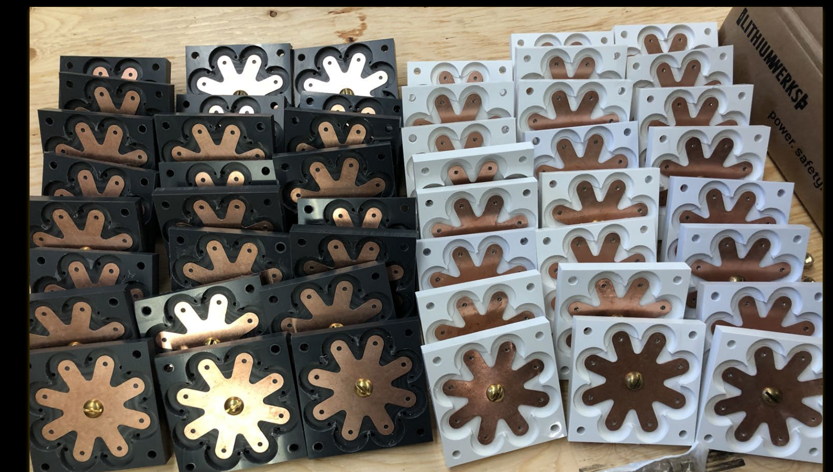
Figure 6: PVC battery caps with copper flowers.
