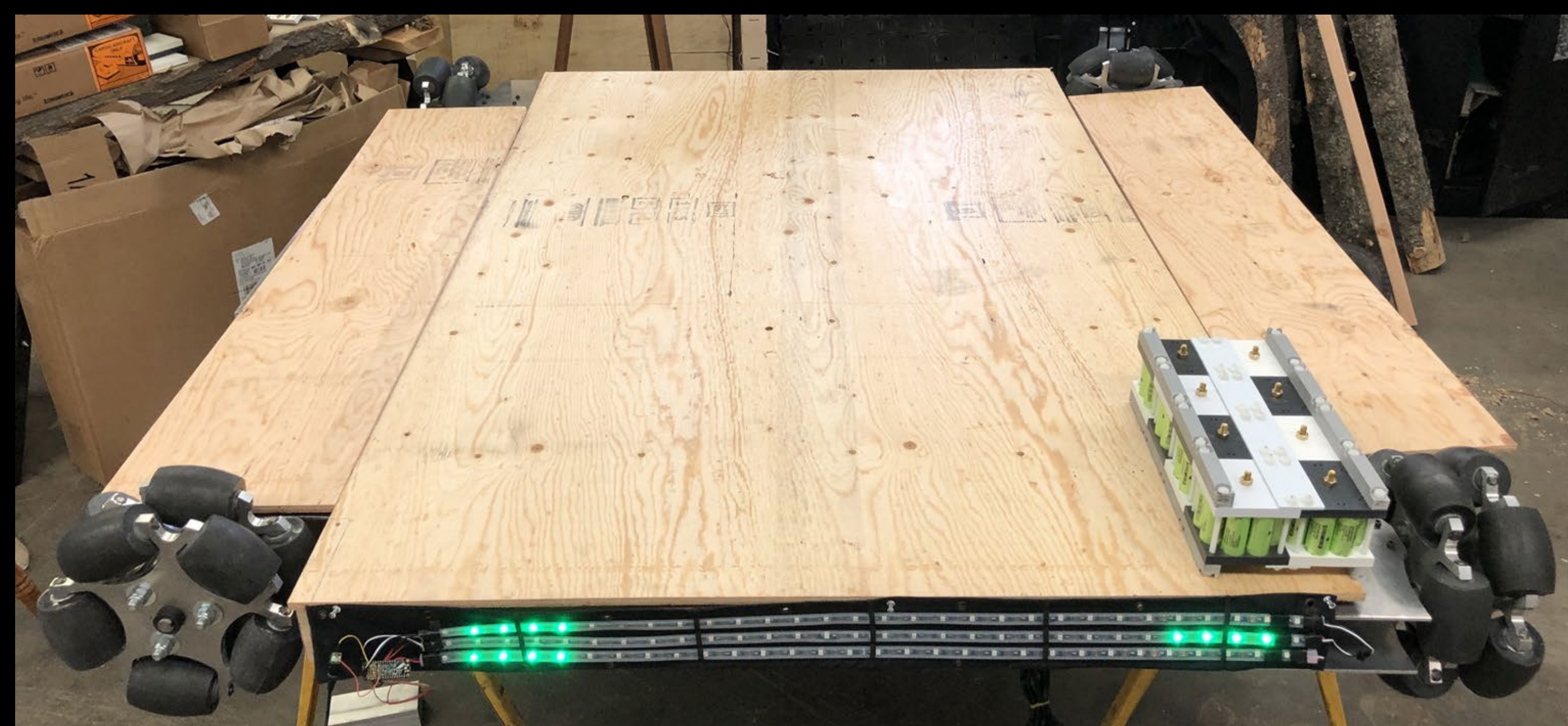
Figure 5: Completed platform, with \frac{1}{2} " plywood decking, one of the four battery packs, and light strip attached. Four remote-controlled, battery-powered LED light strips hang on each side of the platform. Light strips can also be attached to instruments.
