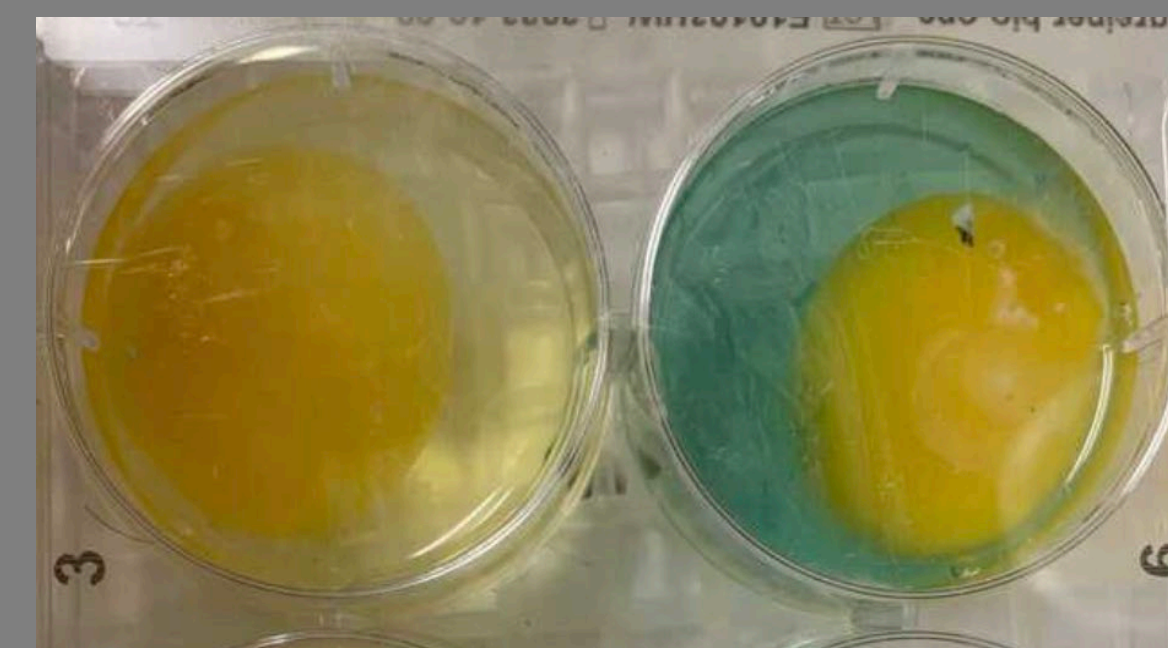
Figure 3: pH dye used in combination with MATLAB to determine pH value.
