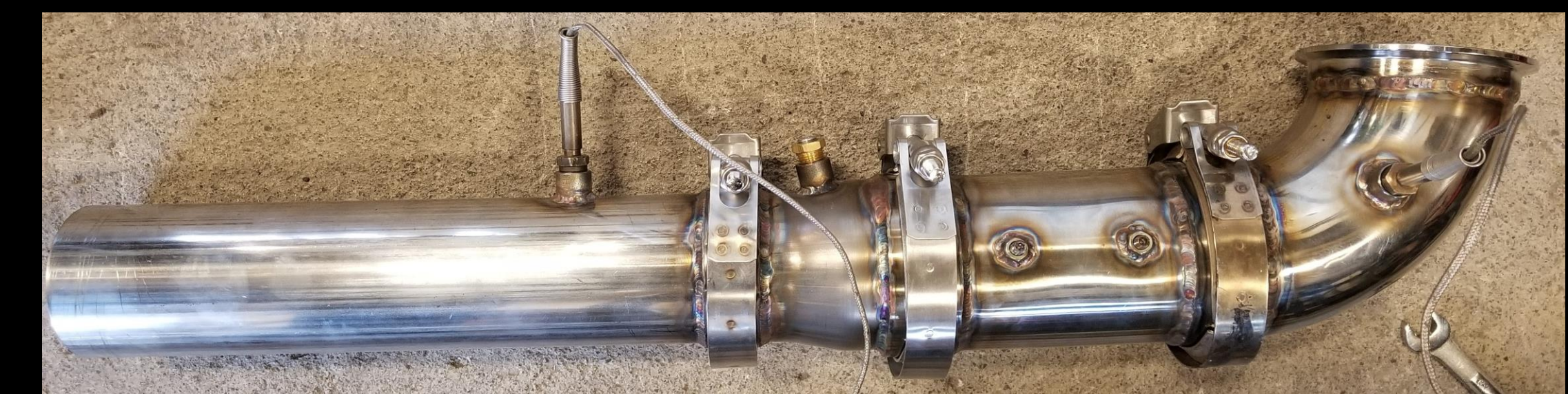
Interchangeable Catalyst Test Pipe
