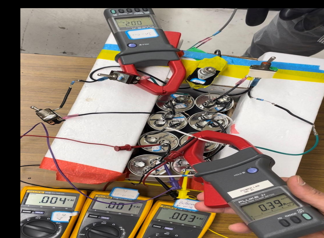
Figure 9: C_1 is shorted, I_{H\text{-bridge}}=0.39A ; I_{C1}=0.02A
