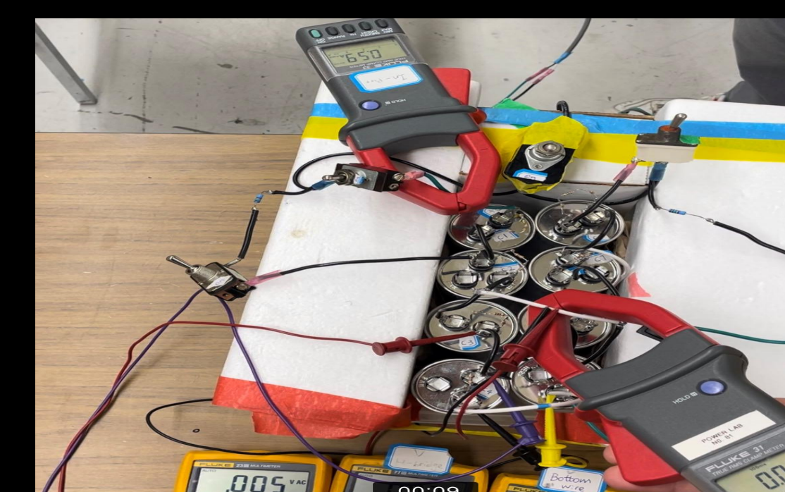
Figure 8: Balanced situation, I_{H\text{-bridge}}=0A ; I_{C1}=0.59A
