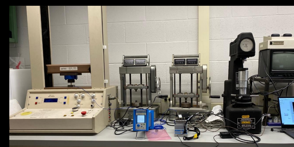
Axial force sensor was calibrated utilizing a load frame shown in above images.
