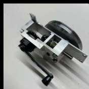
Top view of the gear mech
