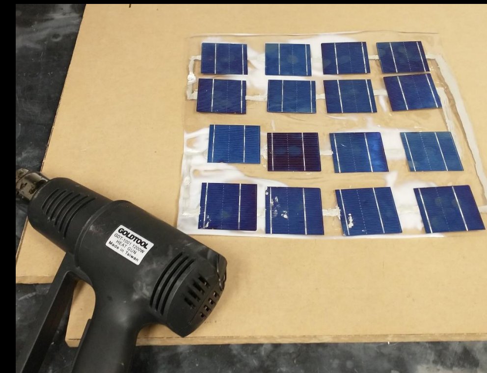
Prototype 1. Fragile Panels, Warping Substrate.
