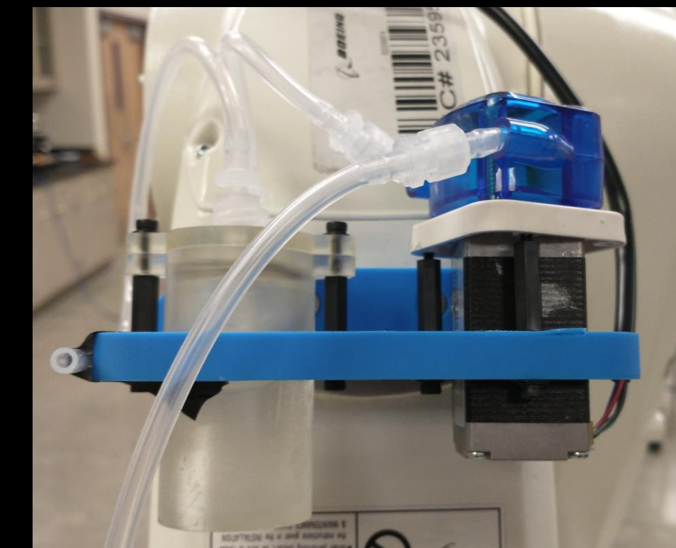
Conductive Ink Reservoir (Resin Printed) and Pump.
