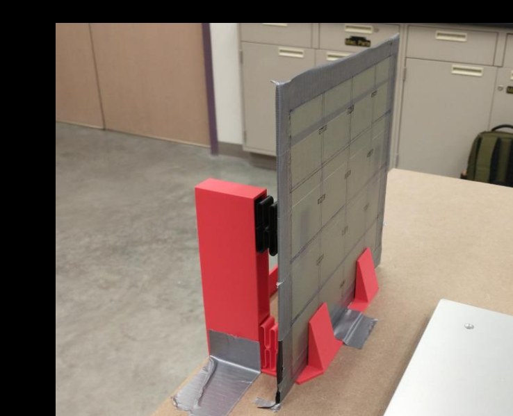
Substrate Dispenser. Uses 3D-Printed Springs. Pictured With Alignment Plate.
