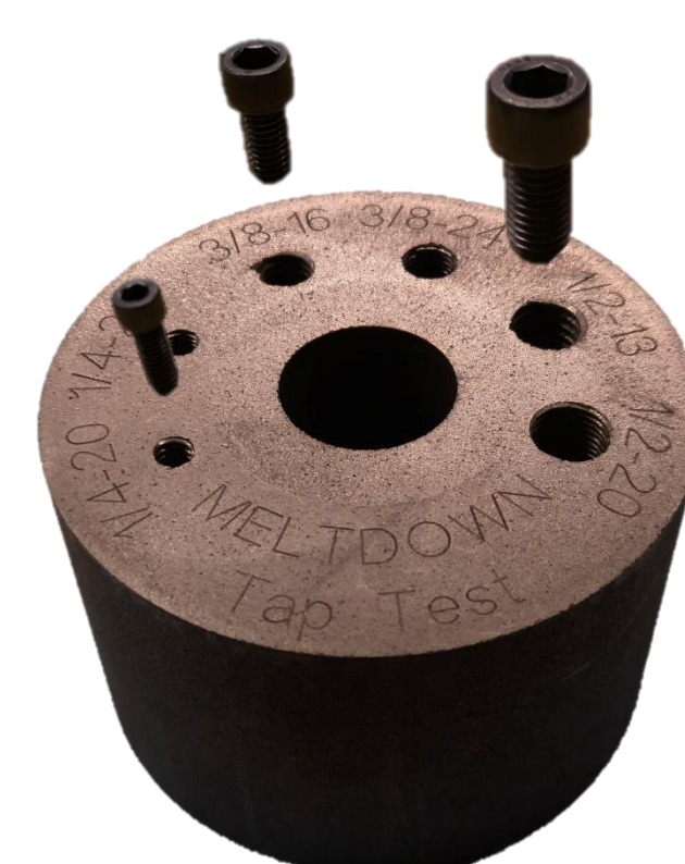
Graphite piece used for thread test
