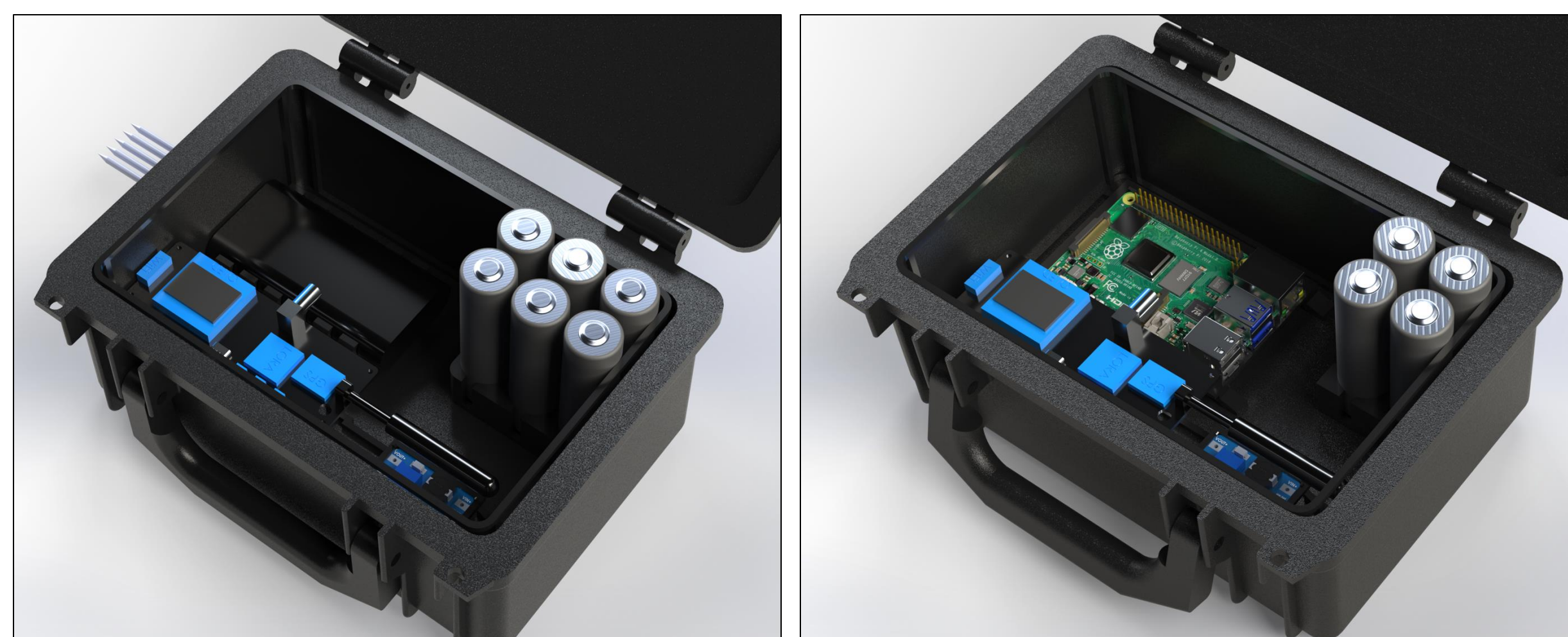
Figure 2: CAD enclosure design UG (left), AG (right)
