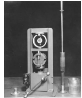
“Marshall method” pavement testing apparatus
