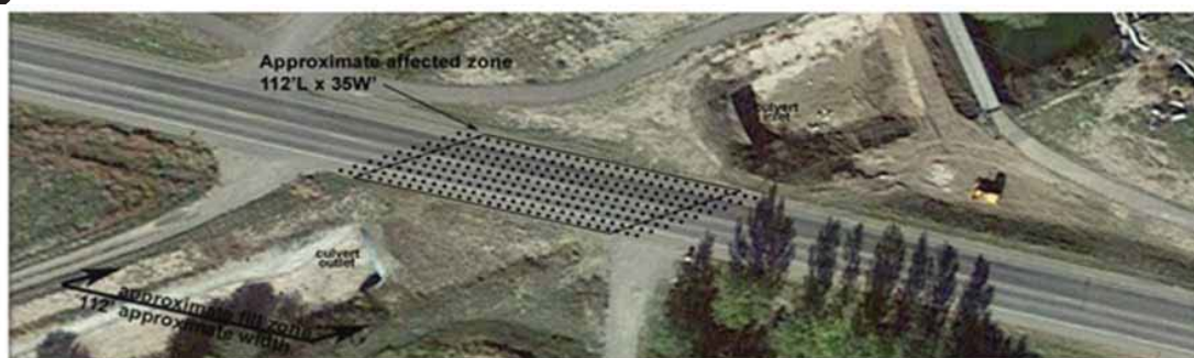
● Approximate Location of Injections, on 4' grid pattern
