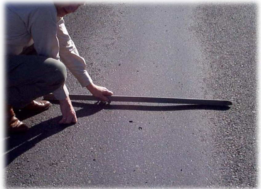
PG 67-22 unmodified, 15mm rut
