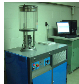
E* Testing using AMPT Machine
