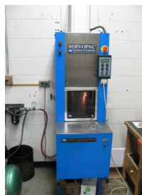
GS Determination from Servopac Gyrotory Compactor data
