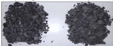
Figure 2 Control RAP mixture (left) and RAP mixture containing GlasPave (right).
