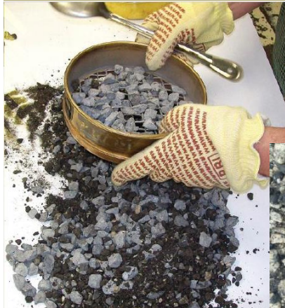
Laboratory heating and blending of 75% virgin aggregate and 25% RAP material
