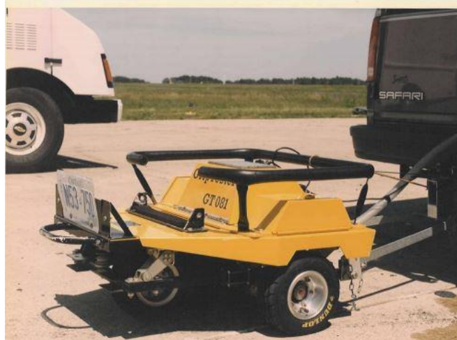
Figure 2-9 Fixed Slip Device (Putov et al. 2016)
