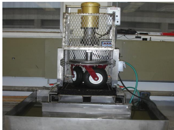
(b) Polishing Test Slabs using TTI polisher
