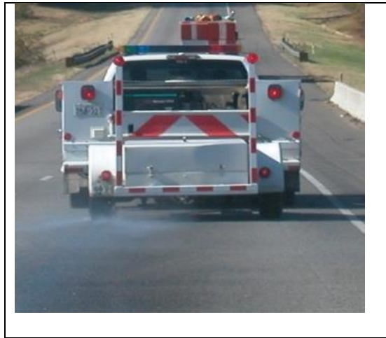
Figure 2-7 Locked-Wheel Skid Trailer
