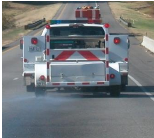
Figure 3-13 Locked-Wheel Skid Trailer
