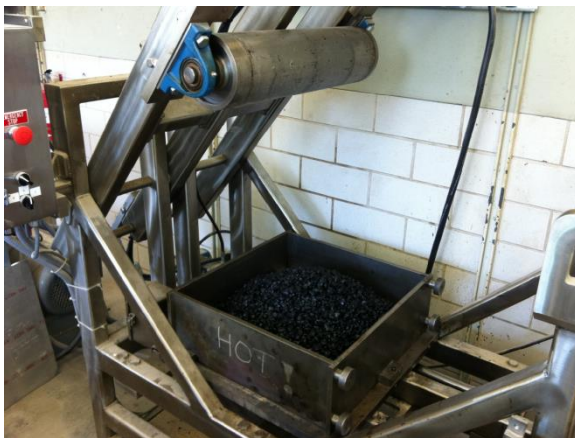
(a) Preparing Slabs using Linear Kneading Compactor
