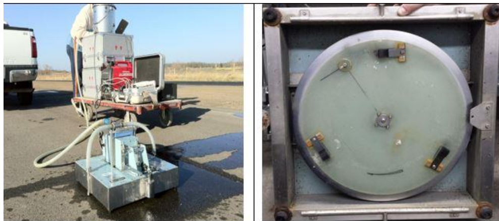
Figure 2-11 Dynamic Friction Tester
