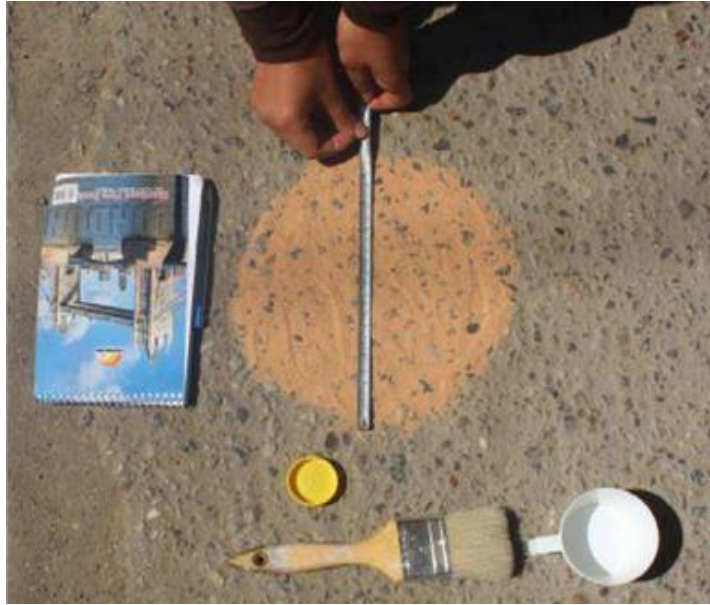
Figure 2-13 Sand Patch Method (Sarsam et al. 2015)
