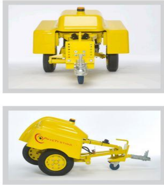
Figure 2-8 Side Force Device (Hall et al. 2009)
