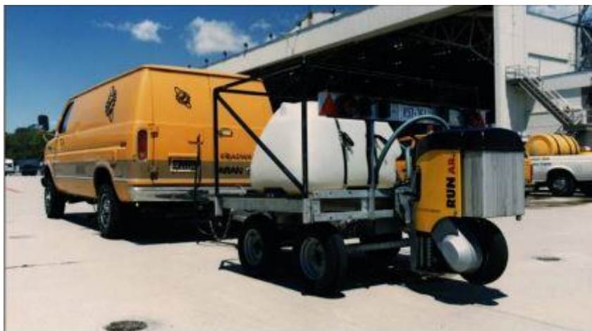
Figure 2-10 Variable Slip Friction Testing Device (Putov et al. 2016)
