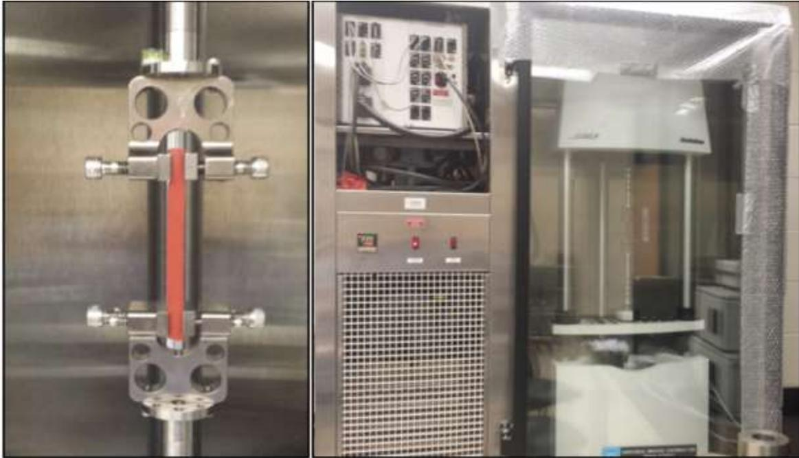
**Figure 2-7.** Testing rubber specimen in the dynamic mechanical analyzer (DMA) device inside a temperature-control chamber
