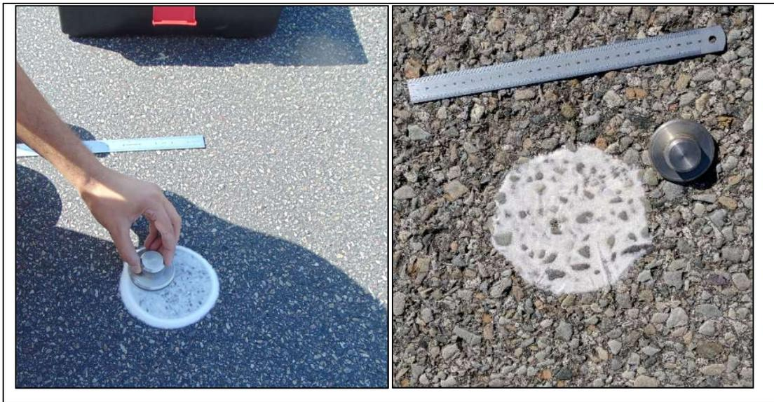
**Figure 3-6.** Typical measurement of pavement macrotexture using the sand patch test
