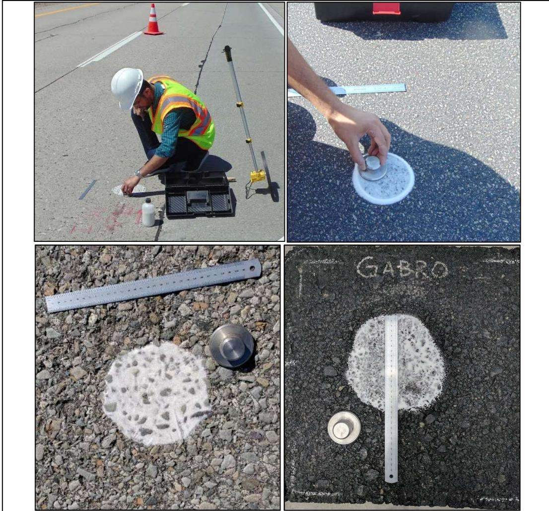
**Figure 4-2.** Measuring pavement macrotexture using the sand patch test.
