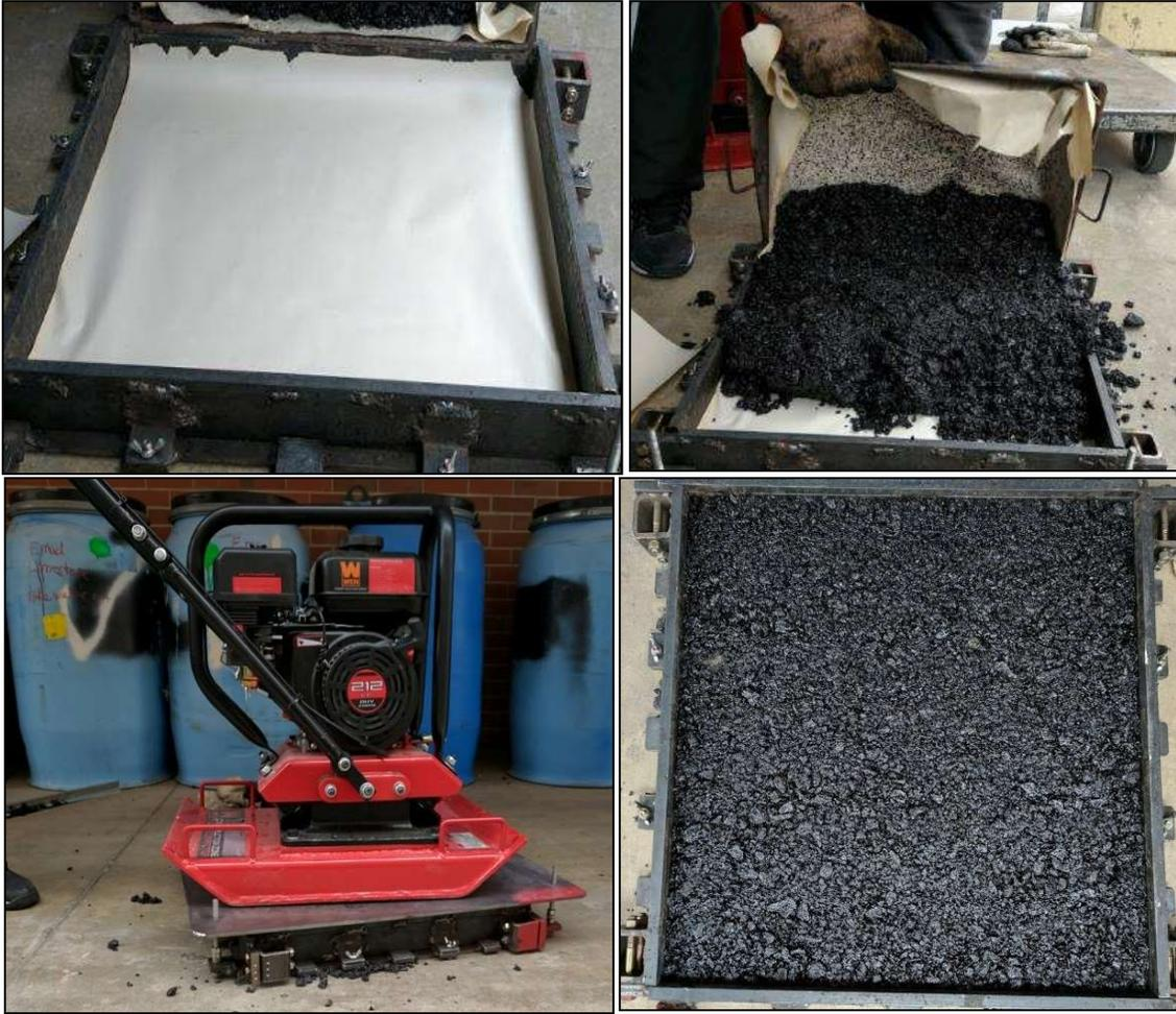
**Figure 2-3.** Preparing hot mix asphalt (HMA) slabs
