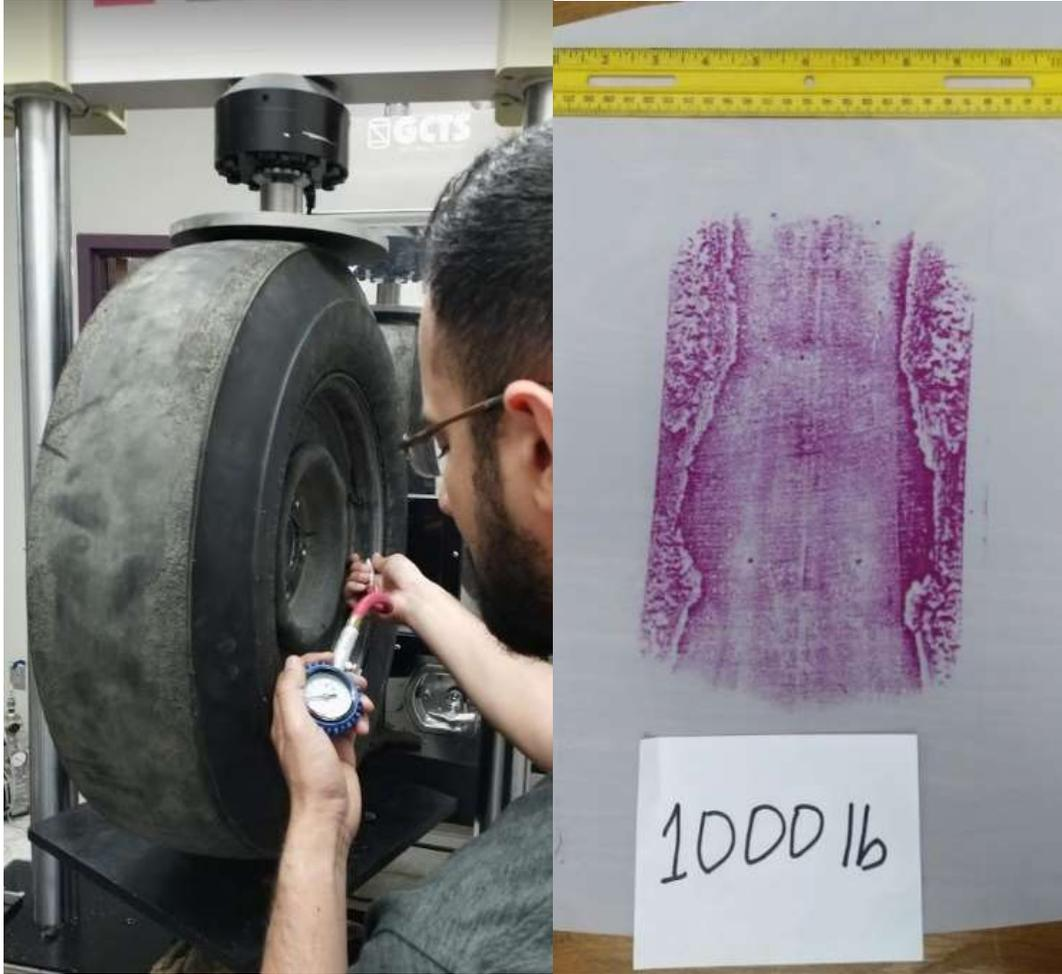
**Figure 5-8.** Measuring the contact area of the ASTM E 524 standard test tire using the MTS machine
