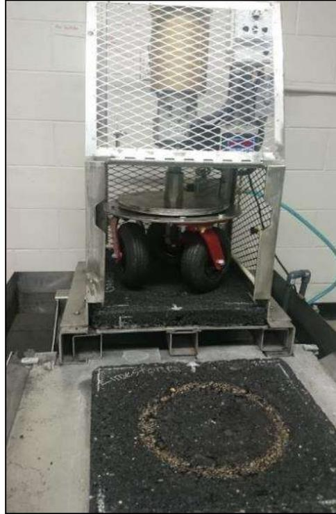
**Figure 2-6.** Three-wheel polisher device
