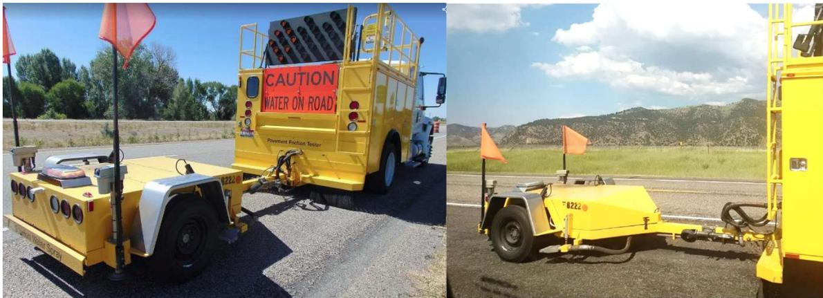
**Figure 4-12.** ITD Pavement Friction Tester
