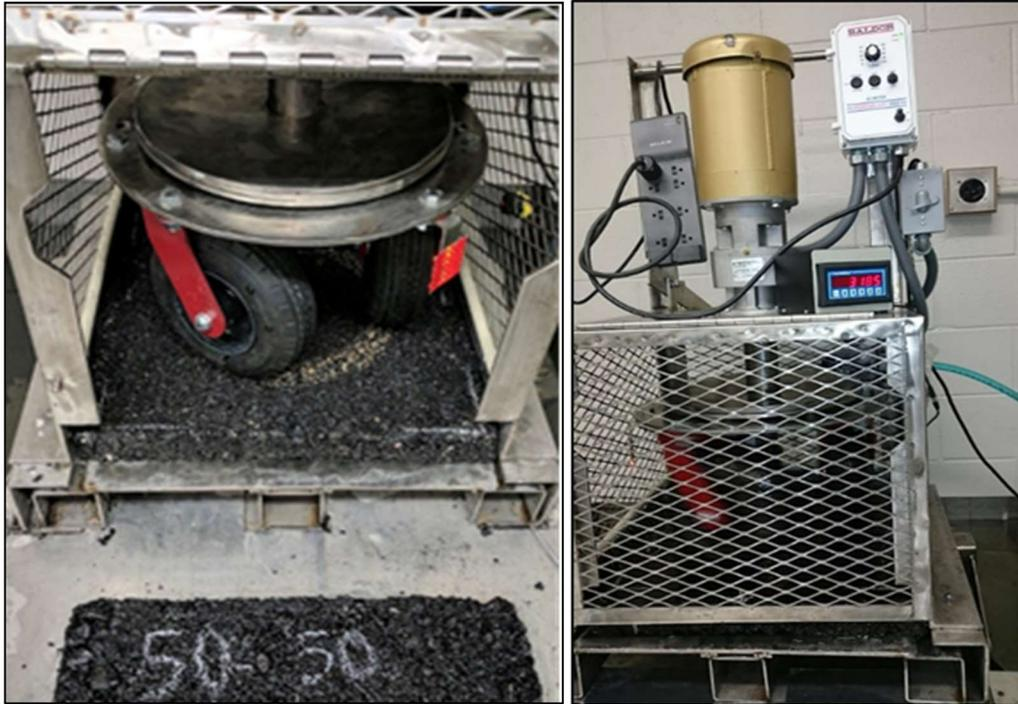
**Figure A-1.** Polishing HMA slabs using the three-wheel polisher
