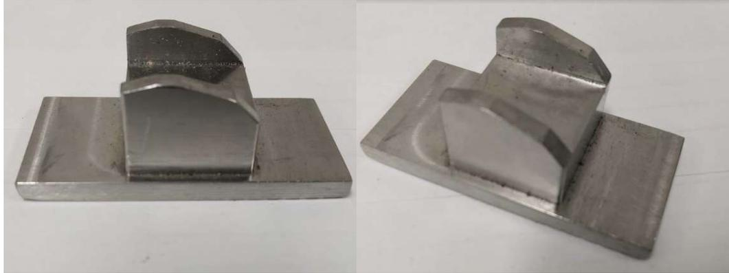
**Figure 4-10.** Metal die used to cut the rubber sliders to the desired shape
