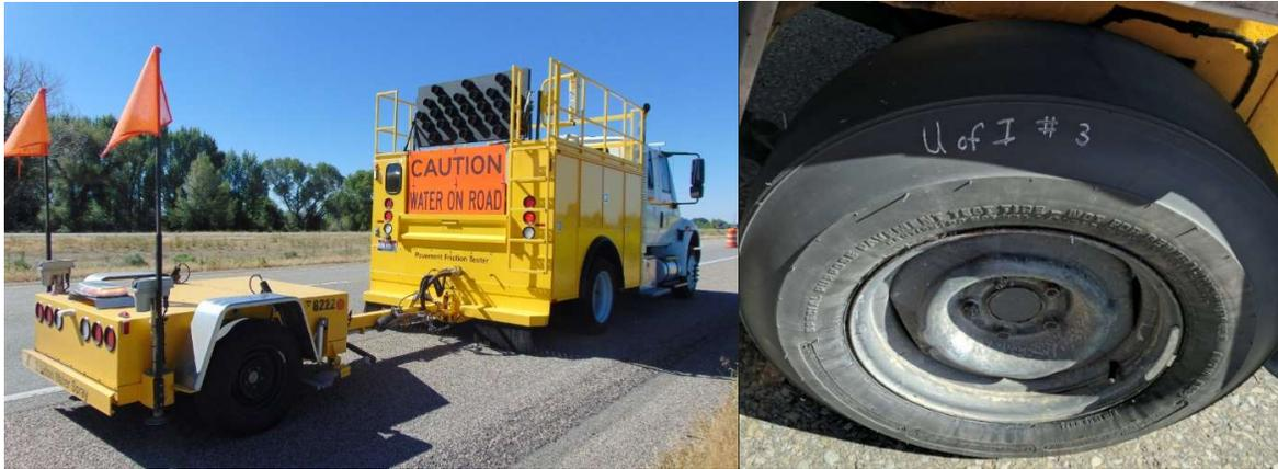
**Figure 3-7.** Locked wheel skid trailer and standard smooth test tire used in Idaho
