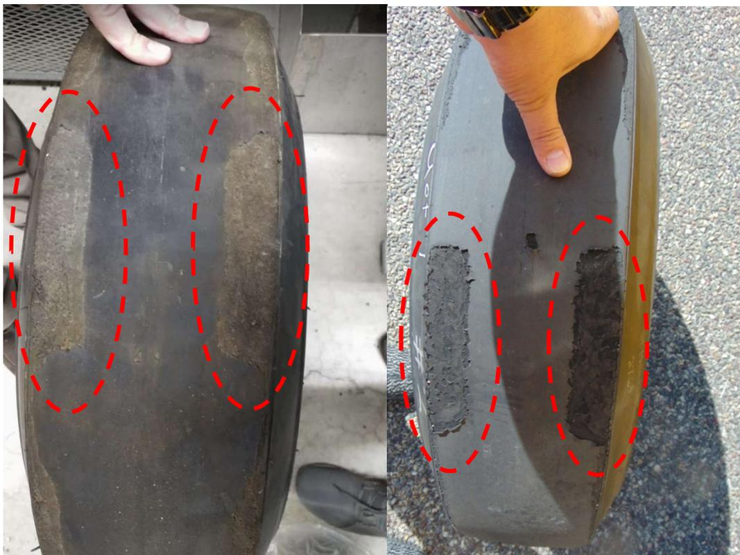
**Figure 5-12.** Wearing pattern of the ASTM E 524 standard test tire
