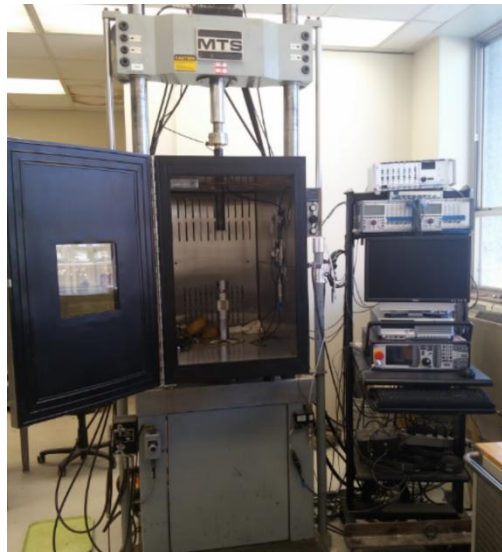
Figure 3.6 the MTS with an Environmental Chamber at the Texas A&M Transportation Institute
