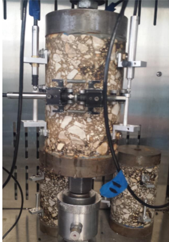
Figure 3.4 Test Setup for the Tension Test
