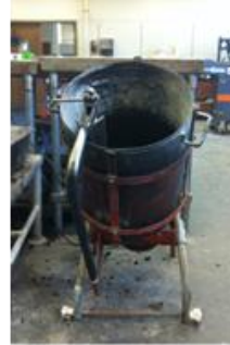
Mixing aggregates with binder
