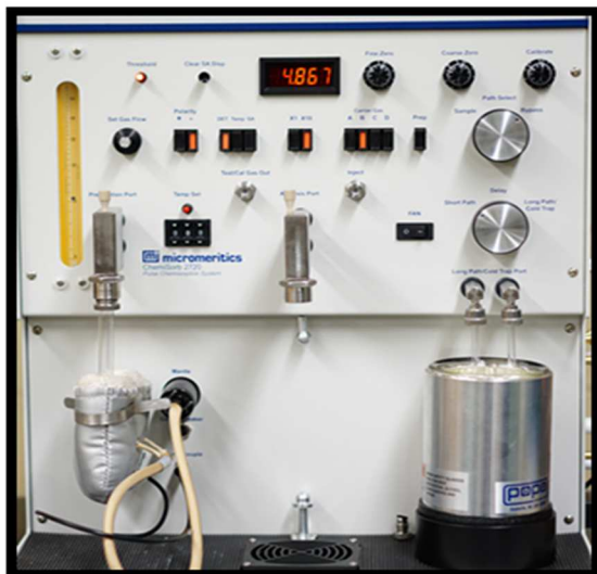
BET analyzer for measuring surface area
