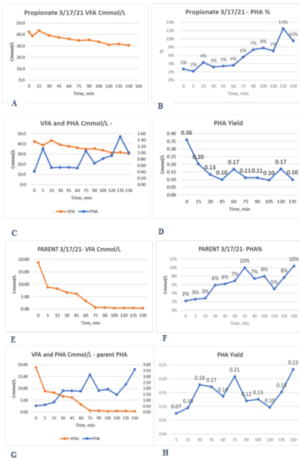
Figure 4.50: Figures A-D belong to the results of the propionate batch-test. Figures E-H are from the parent PHA reactor results (3/17/2021).
