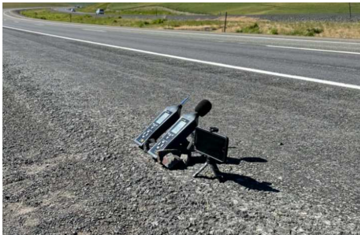
Figure 3.2: Field setup of sound meters (along US-95)
