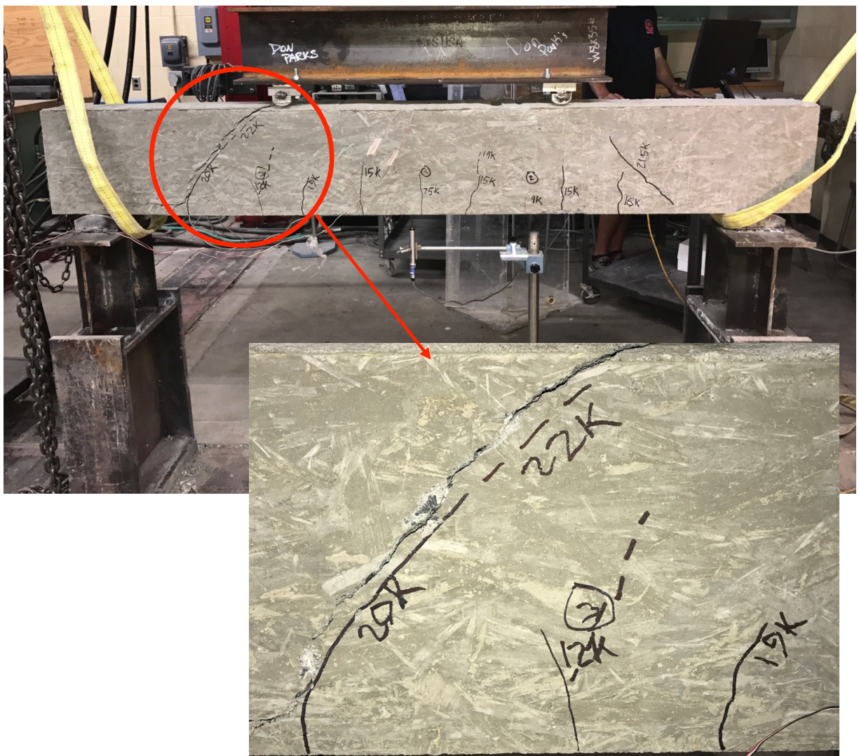
Figure 4.1: Beam 3CONT-MN-2 failure mode (shear failure).
