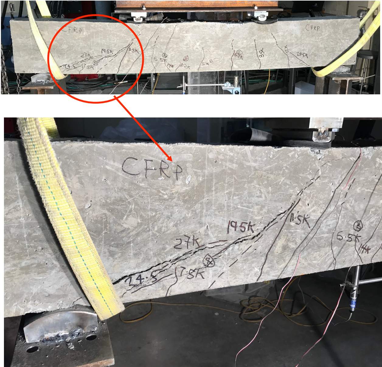
Figure 4.11: Failure mode of 8CF-MN-2.5
