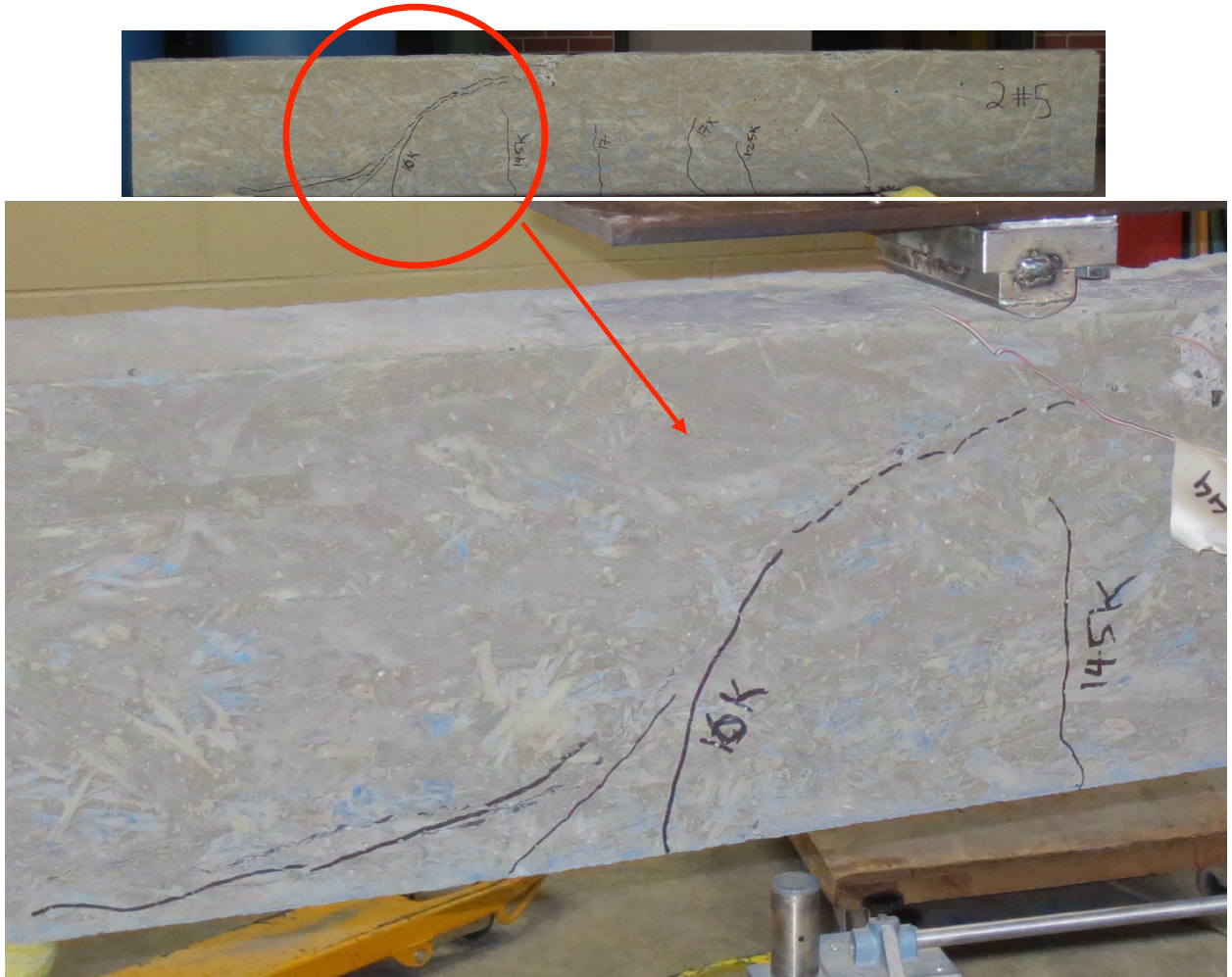
Figure 4.2: Beam 2CONT-MN-2.5 failure mode (shear failure).
