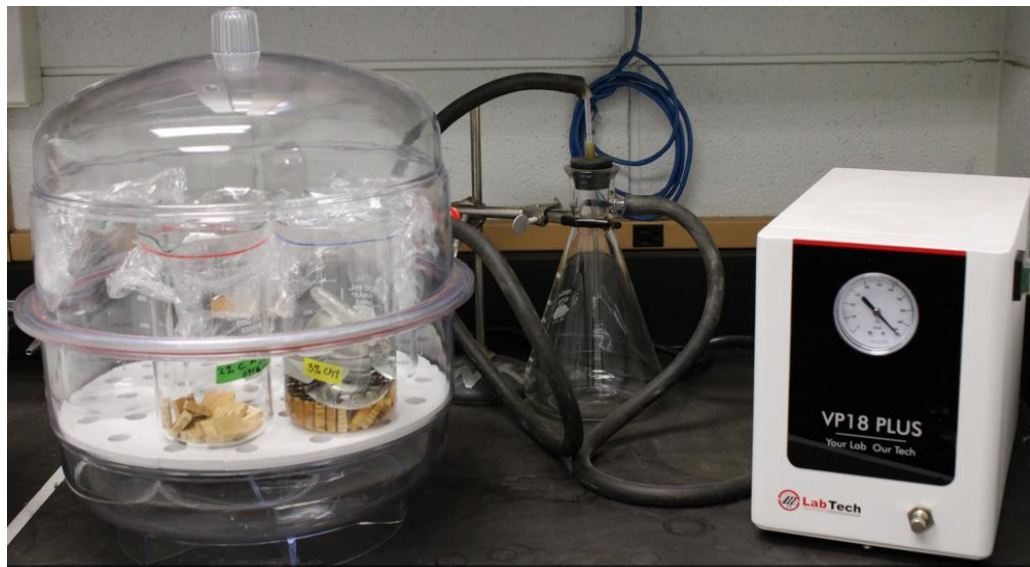
Figure 3. 5: Impregnation of wood with GC precursor solution
