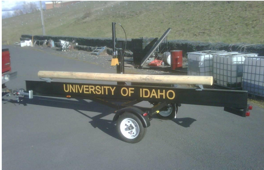
Figure 4. – FlexGrade machine used to perform mid-point testing on small-diameter logs.
