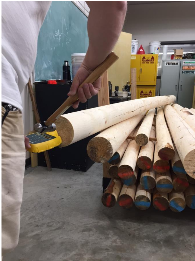
Figure 2. – One of the 6” logs is tested using the Hitman HM200 to measure stress wave velocity.
