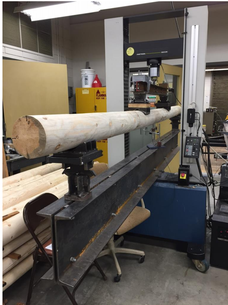
Figure 3. – Instron 5500R machine used for third-point testing to determine static MOE. The 6” log pictured is being tested at the 90° orientation.
