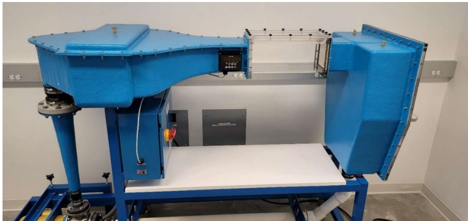
Figure 4.2. 65 Gallon Water Tunnel for Flow Validation Experiments.
