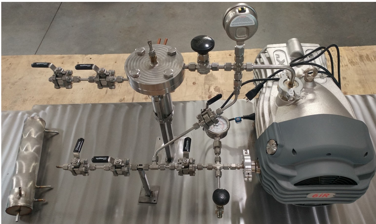
(a) View of the system from the back side while still in the shop. The Ar condenser can be seen on the left, disconnected from the system.
