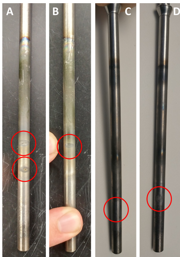
Figure 4.1: Heater rod damage. Both heater rods pictured: Set [A, B] are the first heater rod; set [C, D] are the second. Corrosion and particularly visible damage is circled in red. Additional comments in the text.
