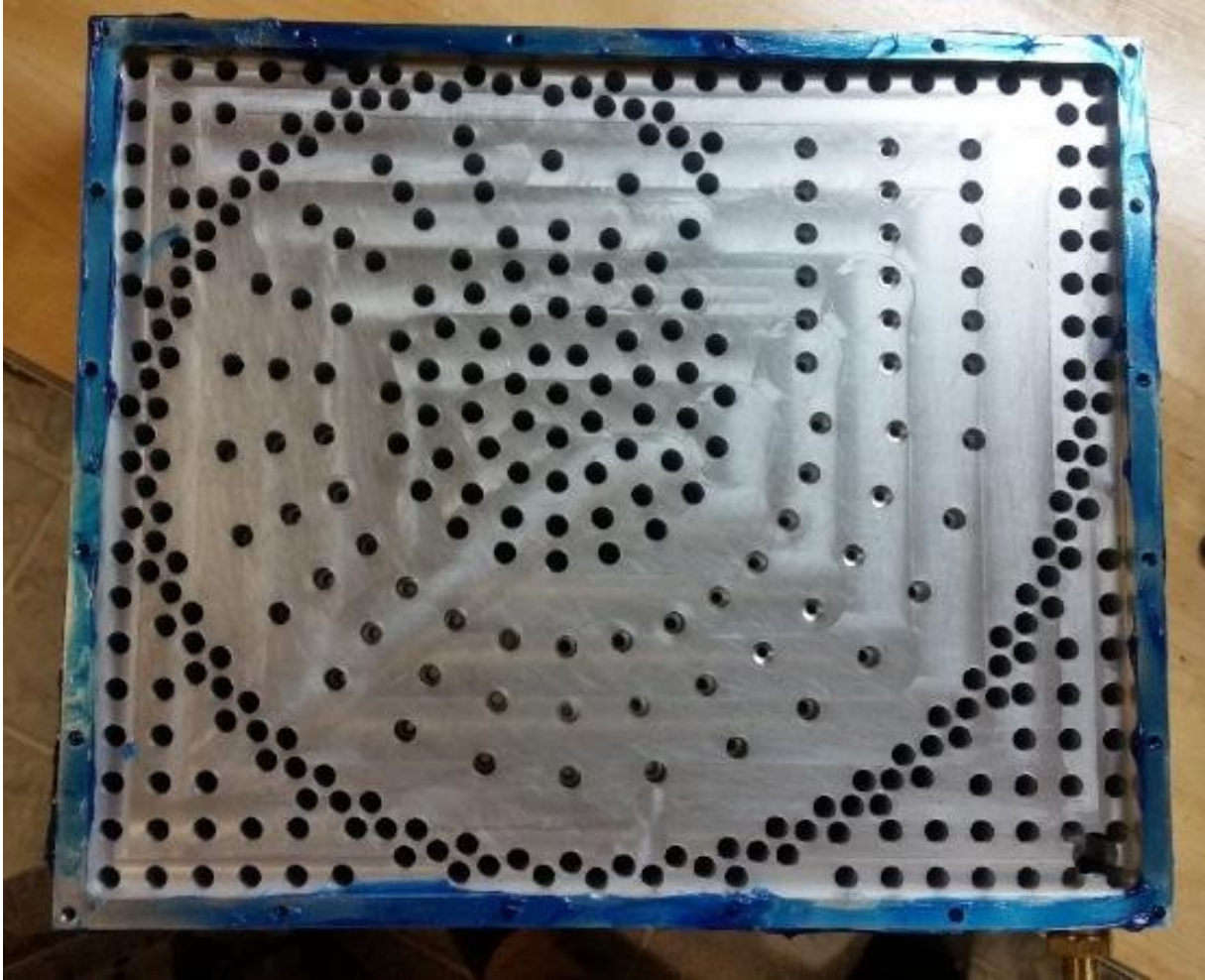
Figure 3.20: An image of the applied grease to form a seal around the outside edge.
