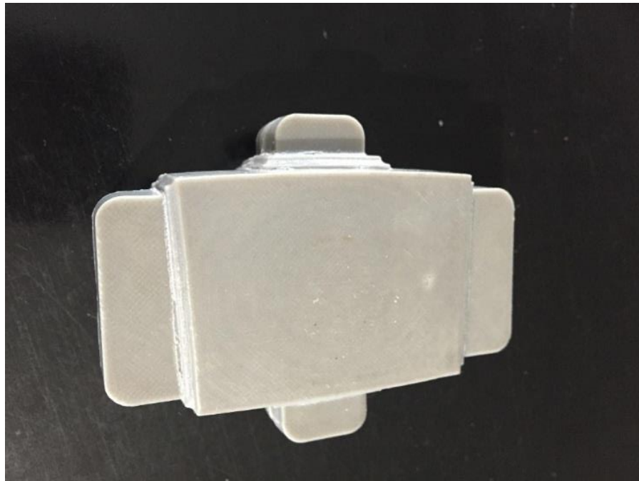
Figure A.2: Acetone smoothed ABS pattern.
