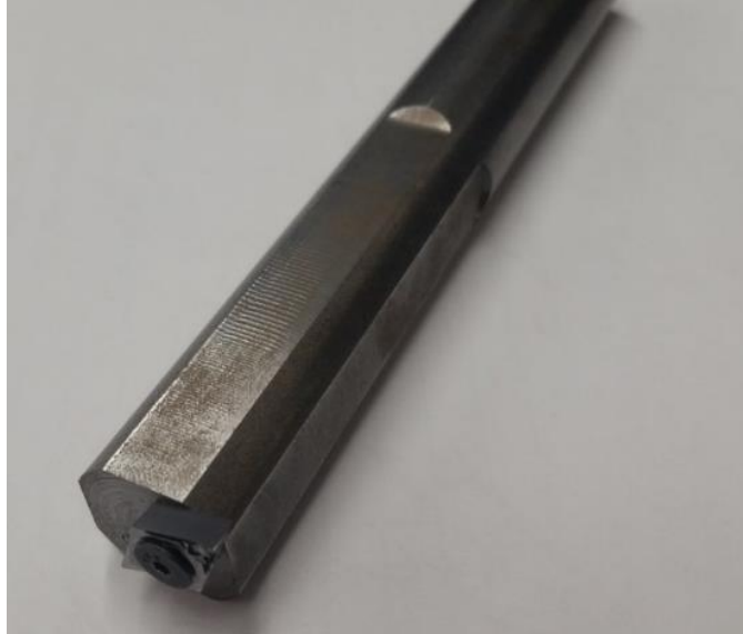
Figure 2.20: Broaching tool used on the internal
