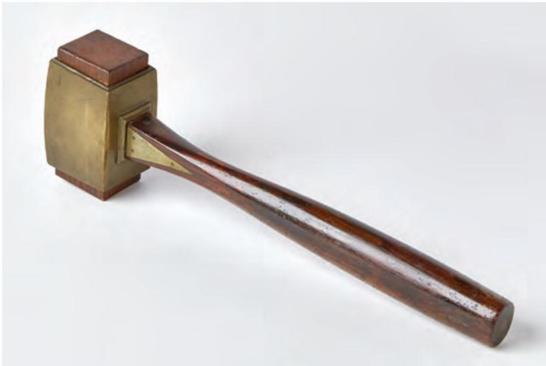
Figure 2.3: Mr. Studley's brass and beech infill mallet. The picture is by Narayan Nayar for use in Williams' book (Williams D. C., 2015).
