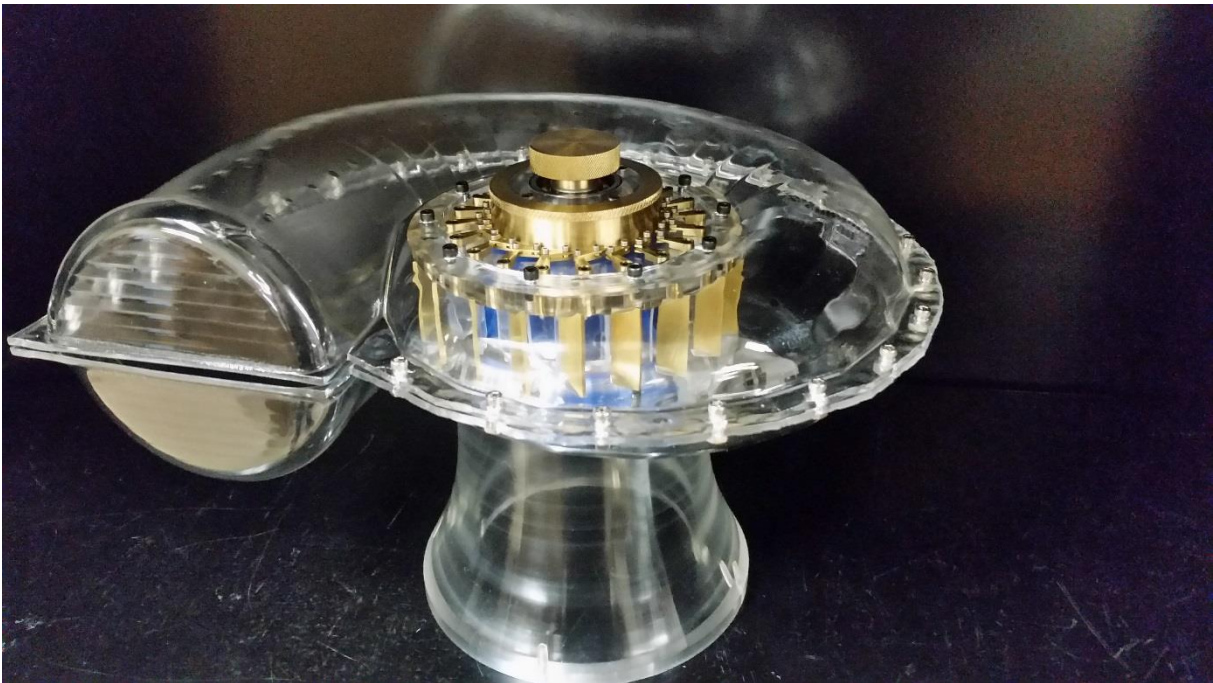
Figure 3.24: An image of the final assembly of the scale model hydroelectric dam.
