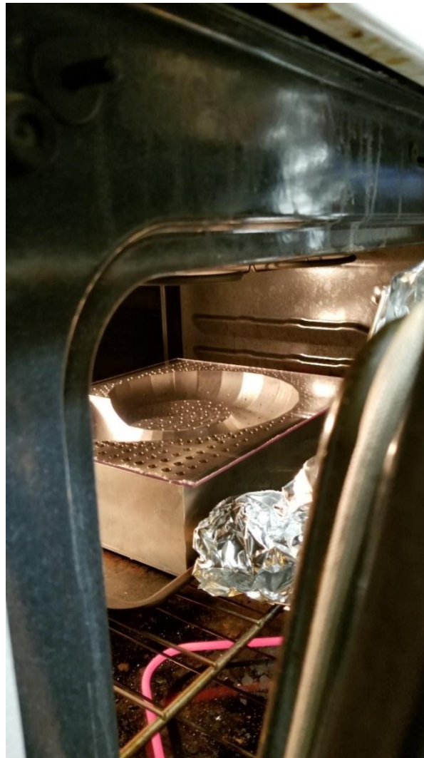
Figure 3.21: Vacuum molding setup in a home oven.
