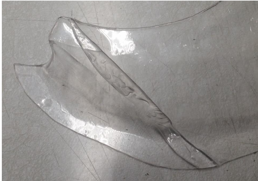
Figure 3.2: an image of the overlapping plastic that occurred during vacuum forming.
