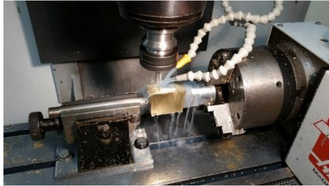
Figure 2.32: An image of the machining process using the 4 th -axis to index the part while machining the shape of the hammer head on each surface.
