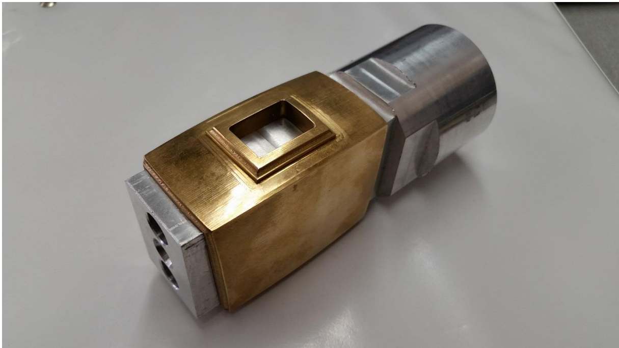
Figure 2.30: An image of the completed virtual 5-axis infill mallet attached to the machining fixture.
