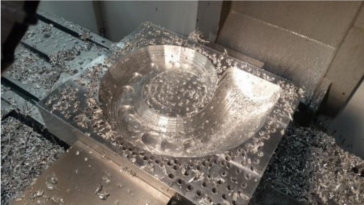
Figure 3.17: An image of one side of the vacuum mold being machined. At this stage the roughing pass of the cavity and finishing pass of the island are complete.
