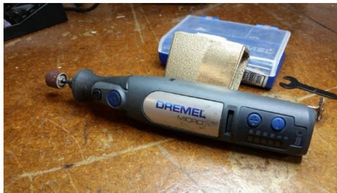
Figure 2.14: Smoothing out have of the first face using a Dremel Micro with a sanding attachment and wire brush.
