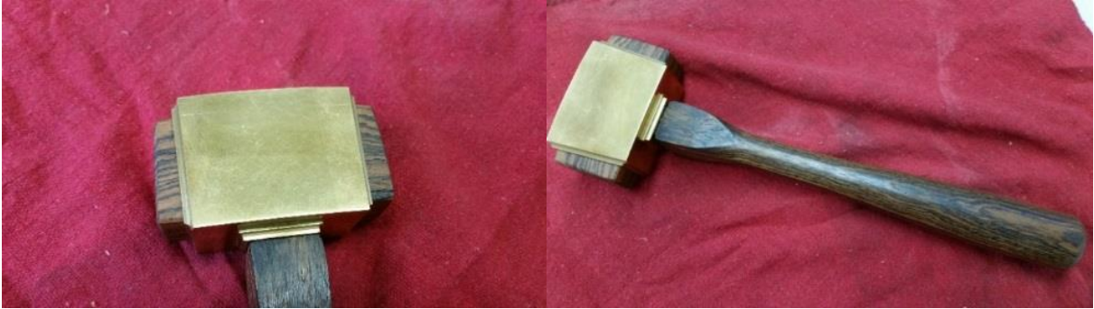
Figure 2.26: Images of the completed 2.5-axis infill mallet with a hardwood infill and handle.
