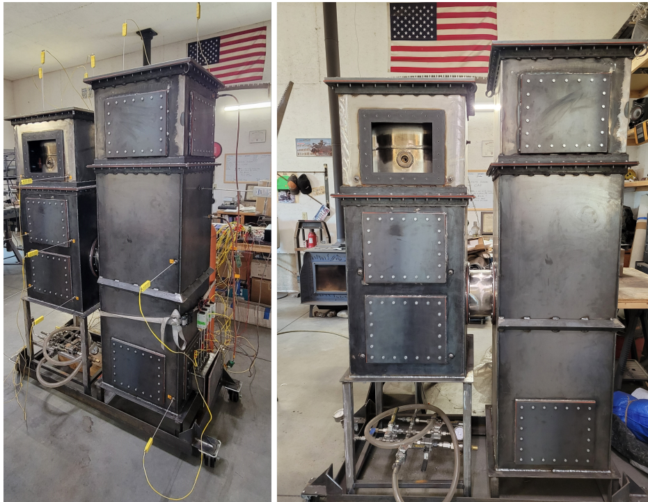
FIGURE 4.2: University of Idaho 1/20 th scaled-down HTGR (front view).
