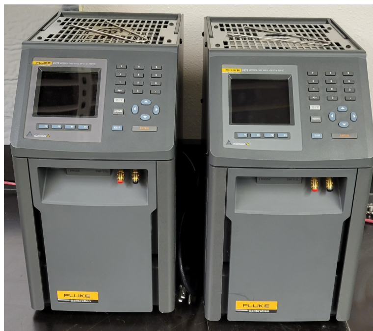
FIGURE 4.20: Fluke 9173 (left) and 9171 (right) thermocouple furnaces.
