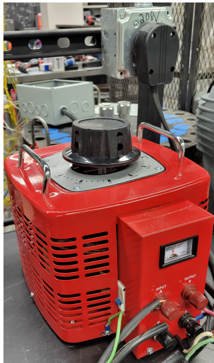
FIGURE 4.8: VEVOR 220V AC variable transformer with dial for output voltage adjustment.
