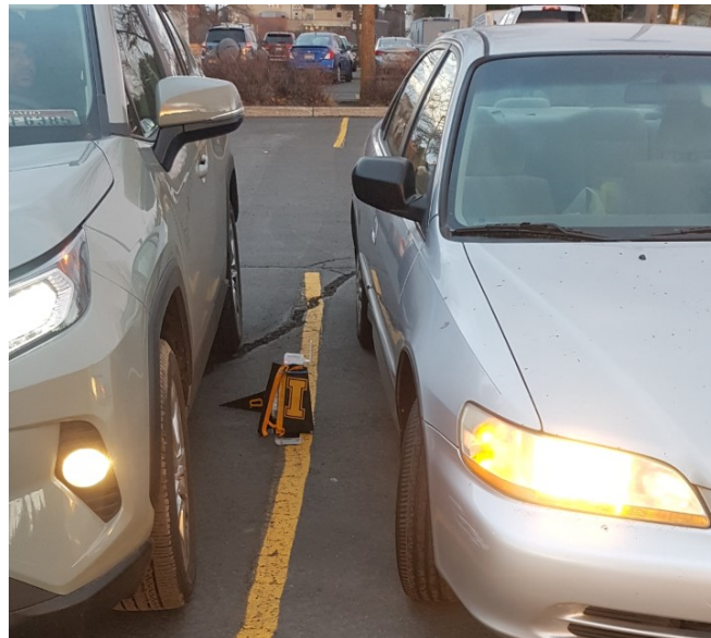
FIGURE 6.10: Low-mounted Locomate ME blocked in between two vehicles
