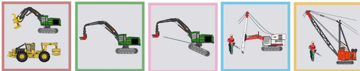
Figure 3.2 Harvest system options for stand classification: feller-buncher/grapple skidder; shovel harvester; tethered-shovel; excavator/ hand fell; swing yarder/ hand fell
