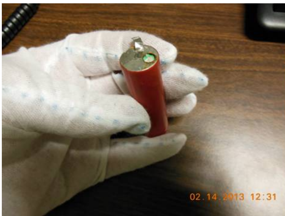
Figure 3.17: Cell with hole cut in the negative end of the can
