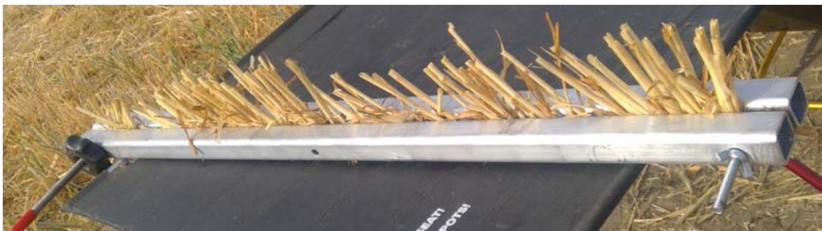
Figure 62: A cell of wheat gripped by the WheatSqueezer version 2, during 2022 testing. Because clamping the cell firmly requires twisting of two nuts on two bolts, the process is slow. Improvements can be made to make mass measurement time-effective.
