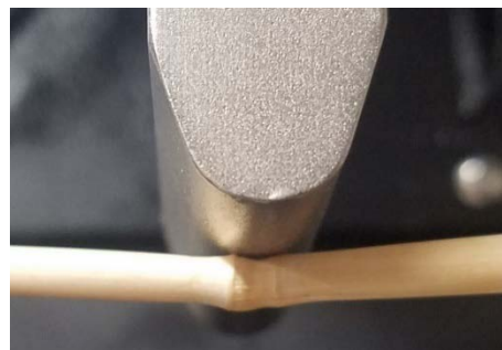
Figure 24: Instron anvil, as used in 2021 trials, in contact with a node of a wheat stem, in the direction of major diameter.
