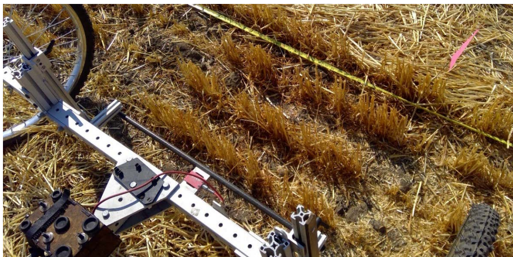
Figure 64: SOCEM lined up for a side hit. Plants have been removed on each side.
