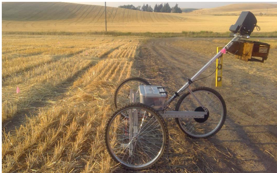
Figure 32: The SOCEM in 2022, prepared for a side hit through a small plot. Improvements include the wooden laser cut keyboard tray, the 3D printed nylon 7" screen housing with attached sunshade, and the removable storage box.
