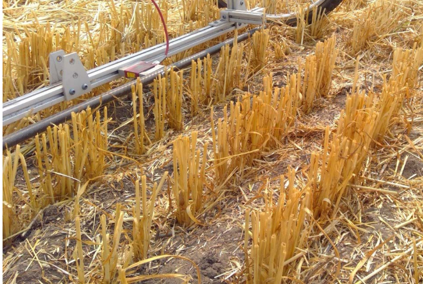
Figure 55: Three rows prepared to be side tested with the SOCEM in 2022. Notice variations in the height of the ground at the base of stems.
