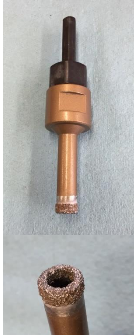
Fig. 4.7 (a) Diamond studded drill ( \text{\O} \frac{1}{2} " DAMO) (b) Drilling into the top of a concrete block using a drill press, process carried out over a plastic tray.
