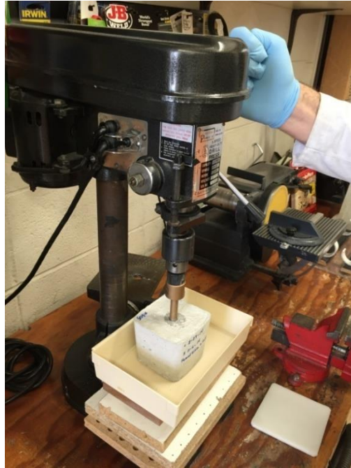
Fig. 4.7 (a) Diamond studded drill ( \text{\O} \frac{1}{2} " DAMO) (b) Drilling into the top of a concrete block using a drill press, process carried out over a plastic tray.
