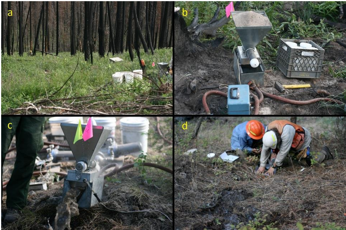
Figure 1.3. Rill experiment images. a) Overview of a rill site; b) Sediment and water mixer with motor controller; c) Sediment and water mixer in operation; d) a sample being taken with a small piece of sheet metal funneling into a collection bottle.
