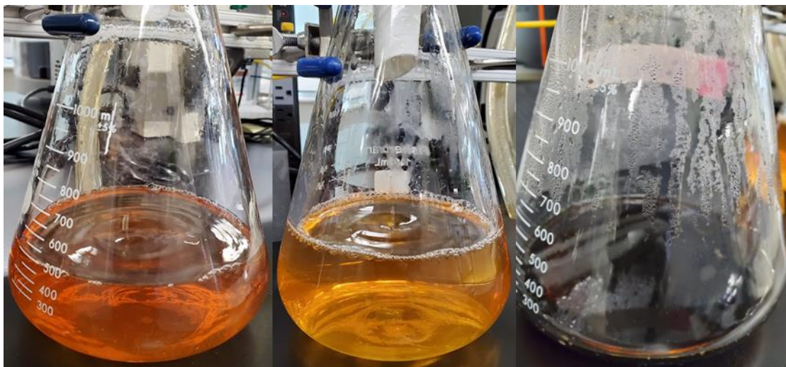
Figure A.2. Filtrate of week 1 bark storage treatments. From left to right: control, 0.1% H 2 SO 4 , and 4% NaOH.
