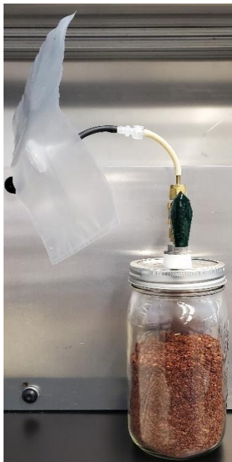
Figure 2.2 Mason jar anaerobic storage pretreatment setup.
