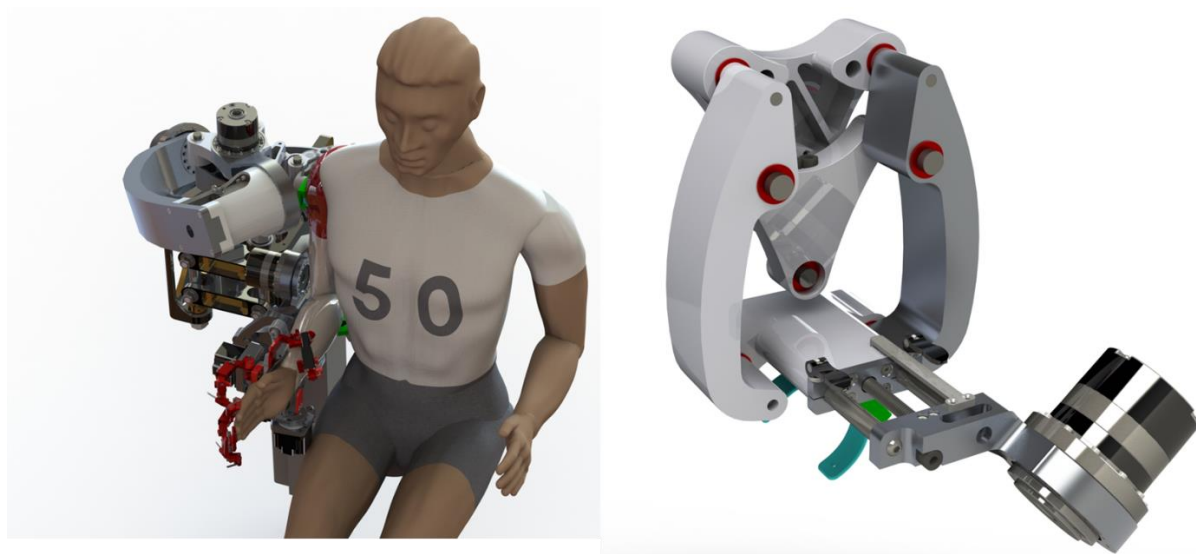
Figure 1-1: A rendering of the right arm of BLUE SABINO and 1005 assembly. The left images illustrates the exoskeleton interacting with a mannequin and the right shows the remote center, parallel-linkage mechanism used for internal/external rotation of the arm.
