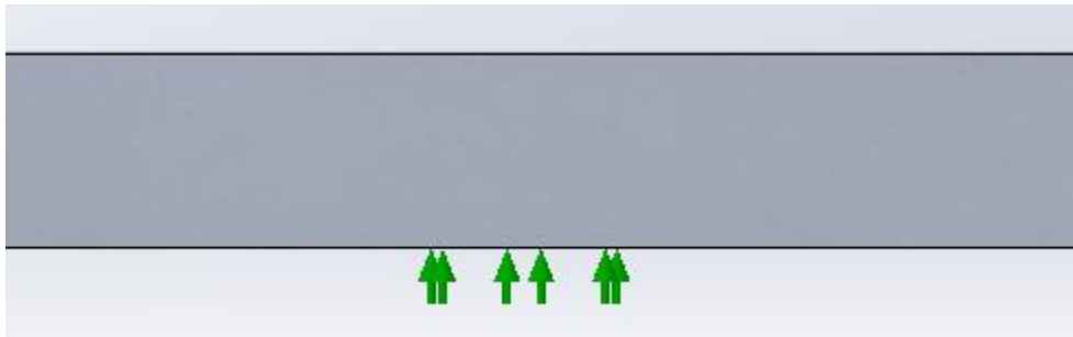
Figure 2-5: An example of a roller/slider fixture being applied to a face within SolidWorks simulation. The green arrows represent the positive direction along with the direction that is being held to zero displacement.
