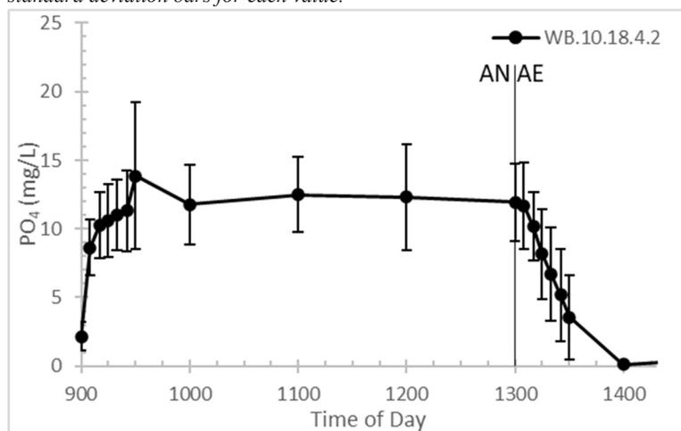
Figure 4.1.4.2: Average PO<sub>4</sub> concentrations in solution for WB.10.18.4.2 with standard deviation bars for each value.
