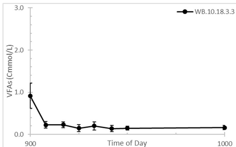
Figure 4.1.3.5: Average VFA concentrations in solution for WB.10.18.3.3 within the first hour of the cycle, including standard deviation bars for each value.
