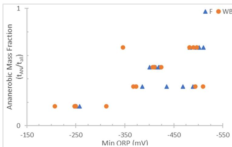
Figure 4.5.1: Minimum anaerobic ORP versus anaerobic mass fraction
