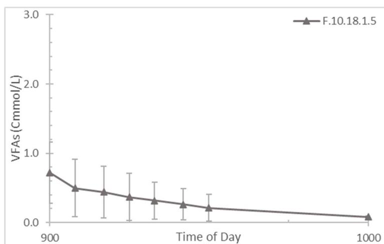
Figure 4.1.1.4: Average VFA concentrations in solution for F.10.18.1.5 within the first hour of the cycle, including standard deviation bars for each value.
