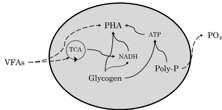
*Figure 2.1.1: Known PAO Metabolisms in the Anaerobic Phase*
