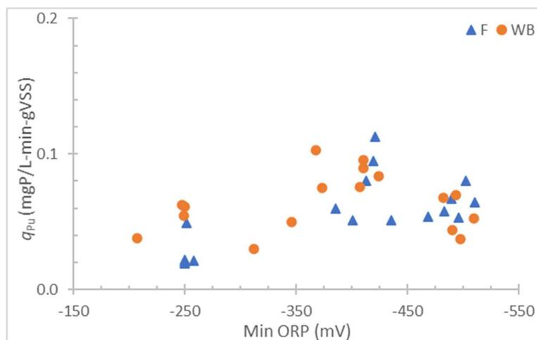
Figure 4.5.1.6: Minimum anaerobic ORP vs specific rate of aerobic  $PO_4$  uptake
