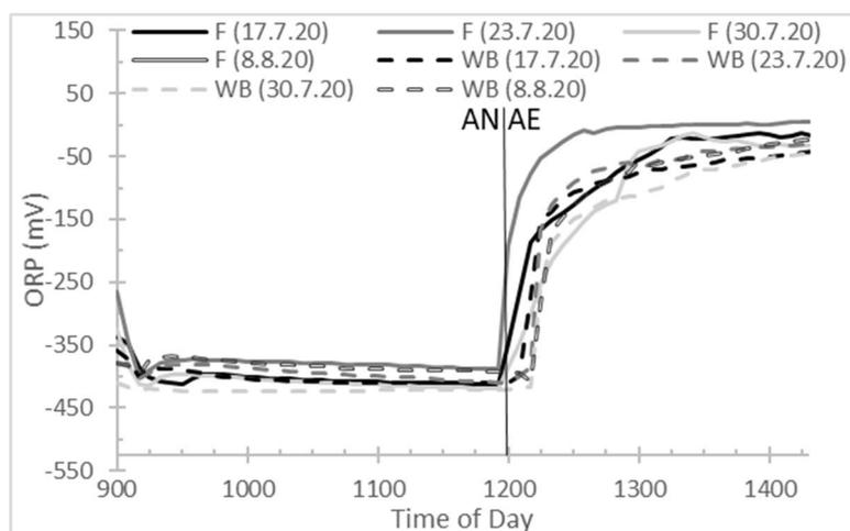
Figure 4.1.3.3: ORP values as measured continuously in solution for F.10.18.3.3 and WB.10.18.3.3 on several dates on which sampling events took place.
