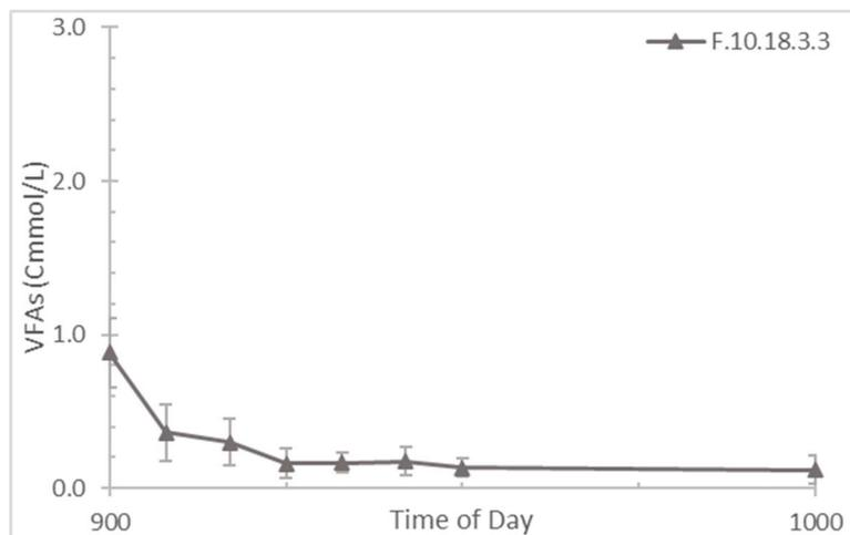
Figure 4.1.3.4: Average VFA concentrations in solution for F.10.18.3.3 within the first hour of the cycle, including standard deviation bars for each value.
