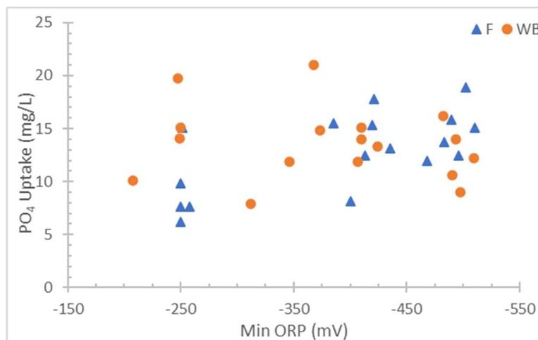
Figure 4.5.1.5: Minimum anaerobic ORP vs total aerobic phosphorus uptake
