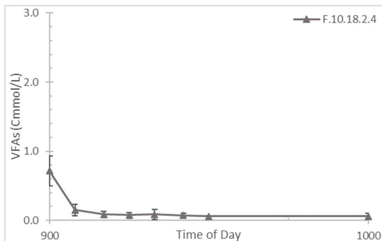
Figure 4.1.2.4: Average VFA concentrations in solution for F.10.18.2.4 within the first hour of the cycle, including standard deviation bars for each value.
