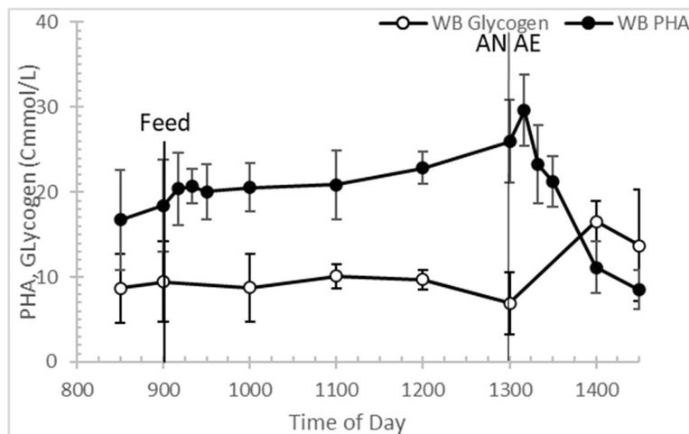
Figure 4.1.4.7: Average Glycogen and PHA concentrations for WB.10.18.4.2 with standard deviation bars for each value.
