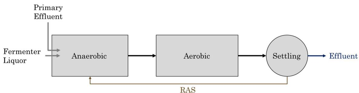
Figure 2.2.1: Flow Diagram for an AO Process
