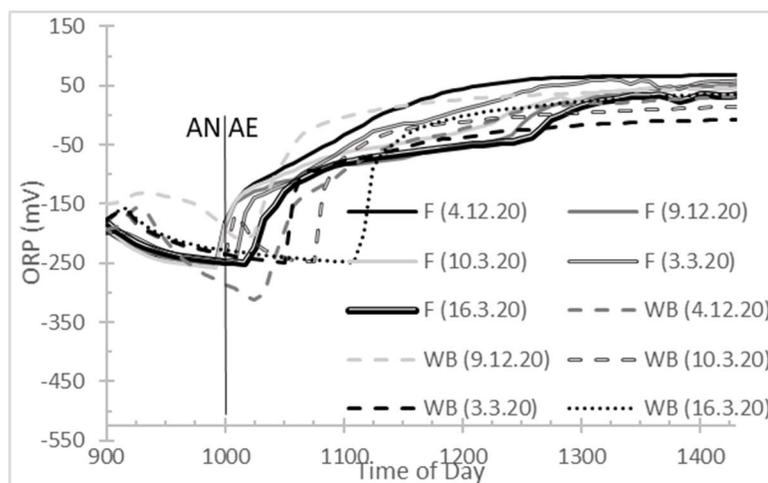
Figure 4.1.1.3: ORP values as measured continuously in solution for F.10.18.1.5 and WB.10.18.1.5 on several dates on which sampling events took place.
