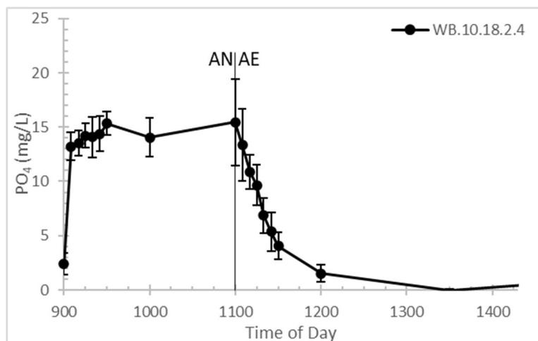
Figure 4.1.2.2: Average  $PO_4$  concentrations in solution for WB.10.18.2.4 with standard deviation bars for each value.
