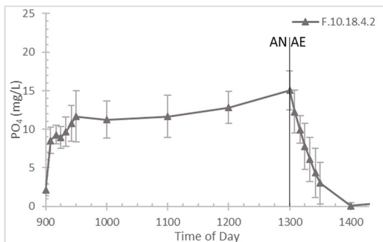
Figure 4.1.4.1: Average PO<sub>4</sub> concentrations in solution for F.10.18.4.2 with standard deviation bars for each value.
