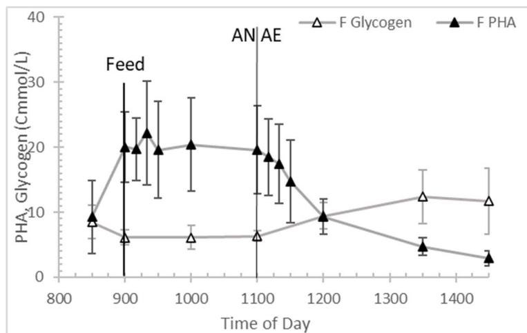
Figure 4.1.2.7: Average Glycogen and PHA concentrations for WB.10.18.2.4 with standard deviation bars for each value.
