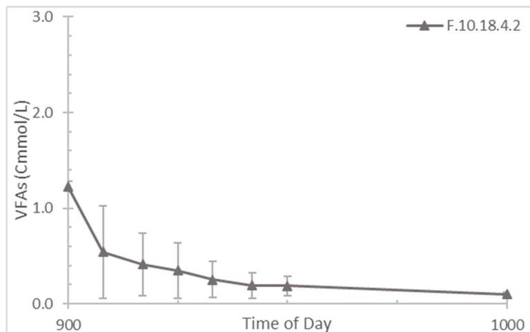
Figure 4.1.4.4: Average VFA concentrations in solution for F.10.18.4.2 within the first hour of the cycle, including standard deviation bars for each value.
