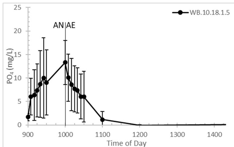
Figure 4.1.1.2: Average  $PO_4$  concentrations in solution for WB.10.18.1.5 with standard deviation bars for each value.
