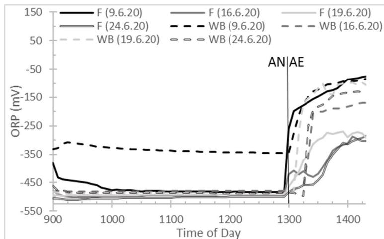
Figure 4.1.4.3: ORP values as measured continuously in solution for F.10.18.4.2 and WB.10.18.4.2 on several dates on which sampling events took place.
