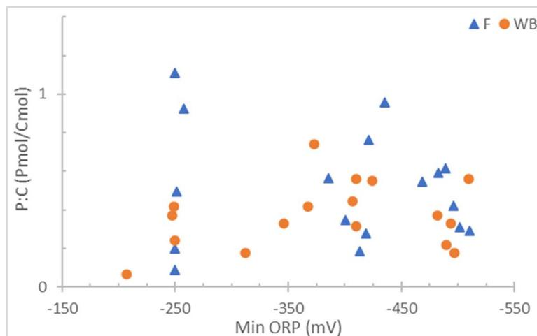
Figure 4.5.2.2: Minimum anaerobic ORP versus anaerobic P:C ratio
