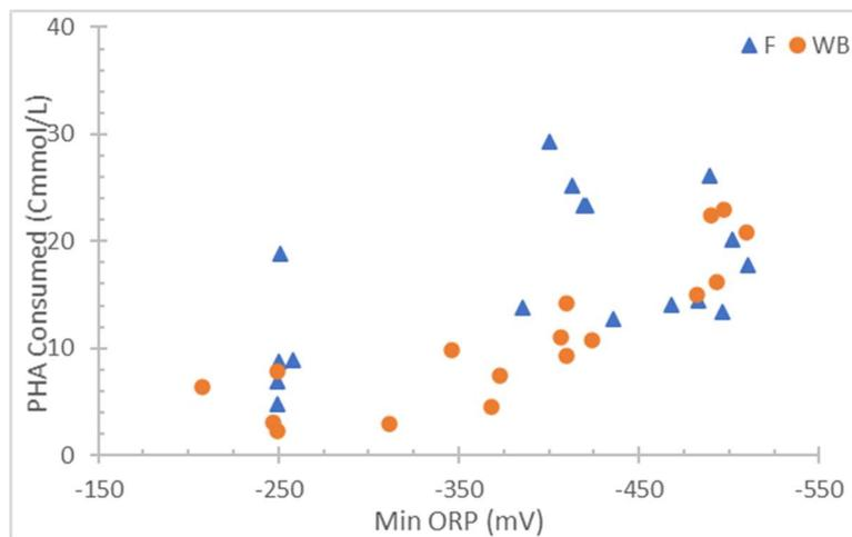
Figure 4.5.3.1: Minimum ORP vs. aerobic PHA consumed
