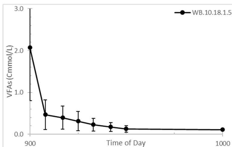
Figure 4.1.1.5: Average VFA concentrations in solution for WB.10.18.1.5 within the first hour of the cycle, including standard deviation bars for each value.
