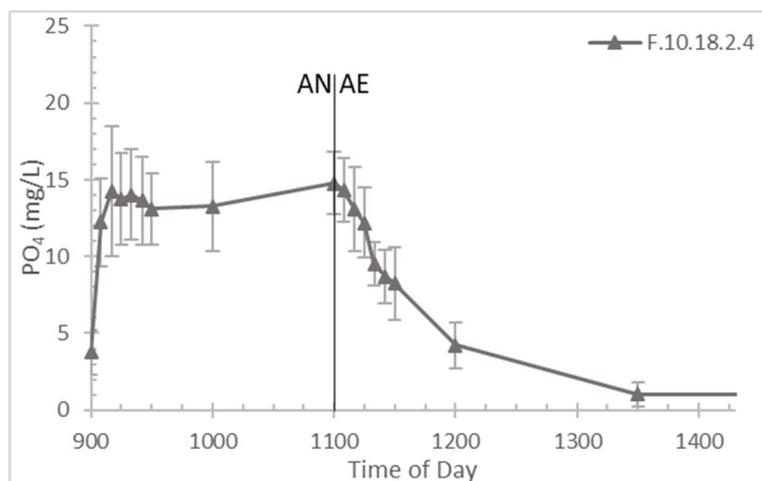
Figure 4.1.2.1: Average  $PO_4$  concentrations in solution for F.10.18.2.4 with standard deviation bars for each value.
