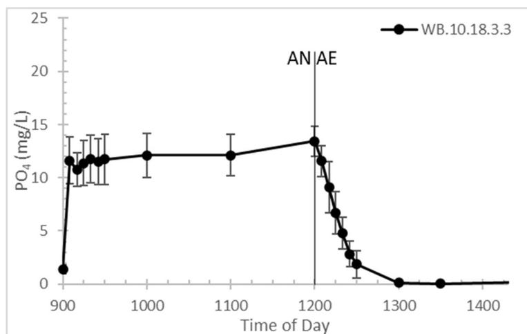
Figure 4.1.3.2: Average PO<sub>4</sub> concentrations in solution for WB.10.18.3.3 with standard deviation bars for each value.
