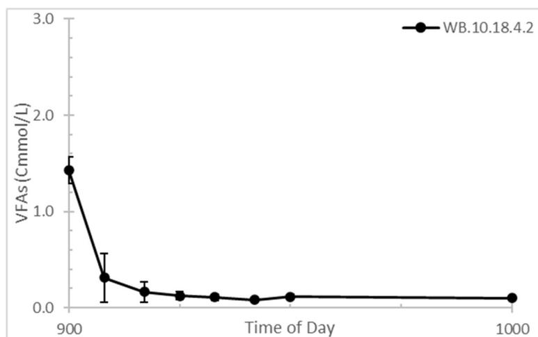
Figure 4.1.4.5: Average VFA concentrations in solution for WB.10.18.4.2 within the first hour of the cycle, including standard deviation bars for each value.
