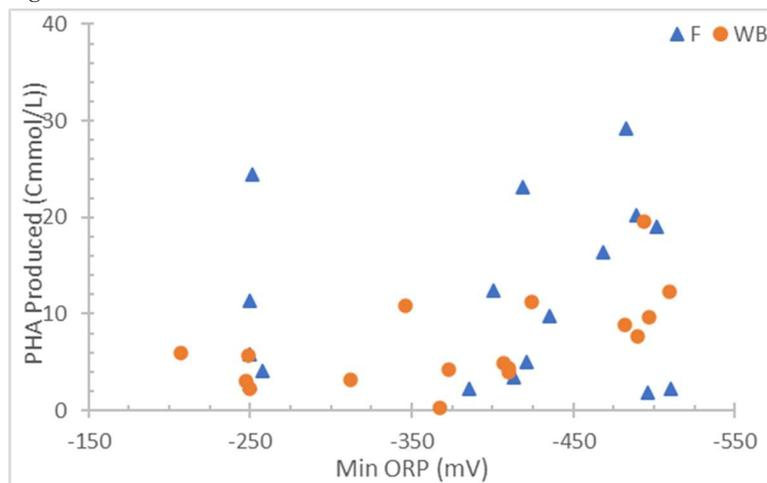
Figure 4.5.3.2: Minimum ORP vs. anaerobic PHA produced
