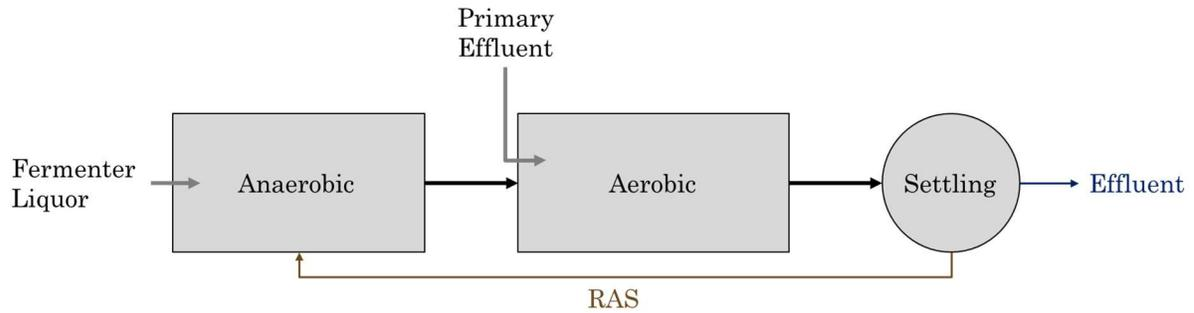
Figure 2.2.2: Flow Diagram for a Westbank Process
