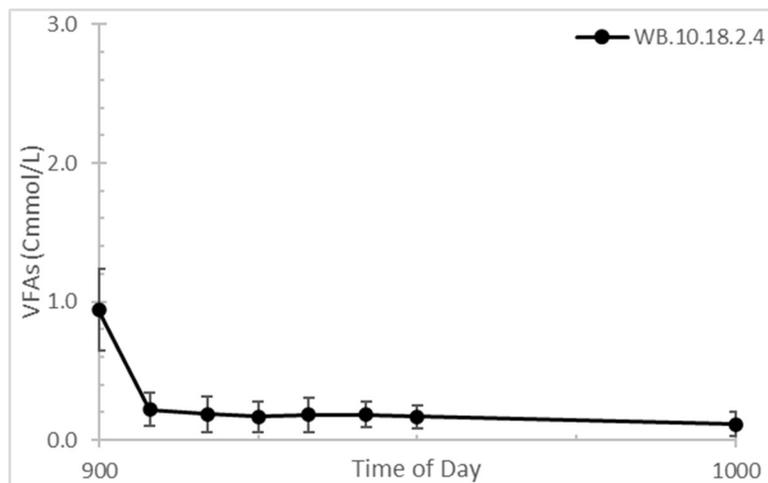
Figure 4.1.2.5: Average VFA concentrations in solution for WB.10.18.2.4 within the first hour of the cycle, including standard deviation bars for each value.
