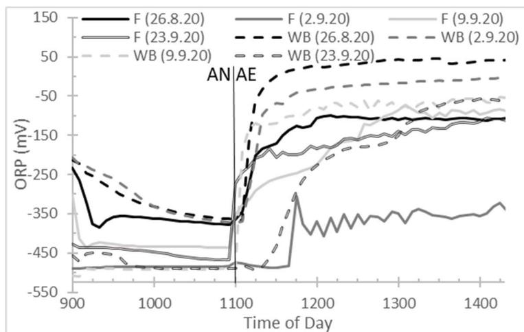
Figure 4.1.2.3: ORP values as measured continuously in solution for F.10.18.2.4 and WB.10.18.2.4 on several dates on which sampling events took place.
