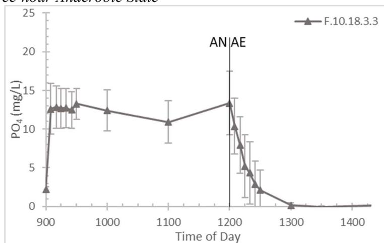
Figure 4.1.3.1: Average PO<sub>4</sub> concentrations in solution for F.10.18.3.3 with standard deviation bars for each value.
